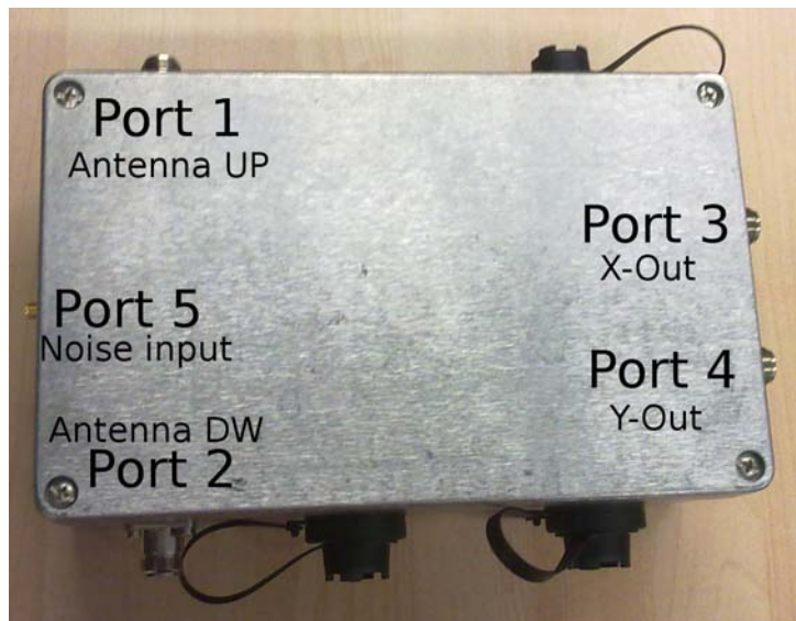
Figure 7.11: External view of the RF front-end and calibration subsystem.
