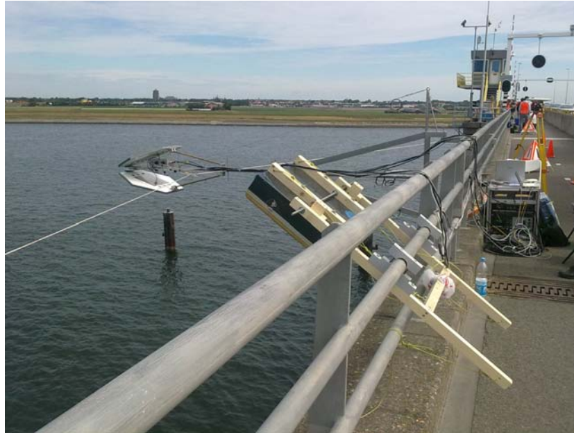
Figure 7.12: Measurement setup at the Zeelandbrug bridge: There is the L-band radiometer in first term, and the GNSS-R antennas' mast behind it. The RADAC instrument was mounted near the bridge's control tower observed at the picture's background
