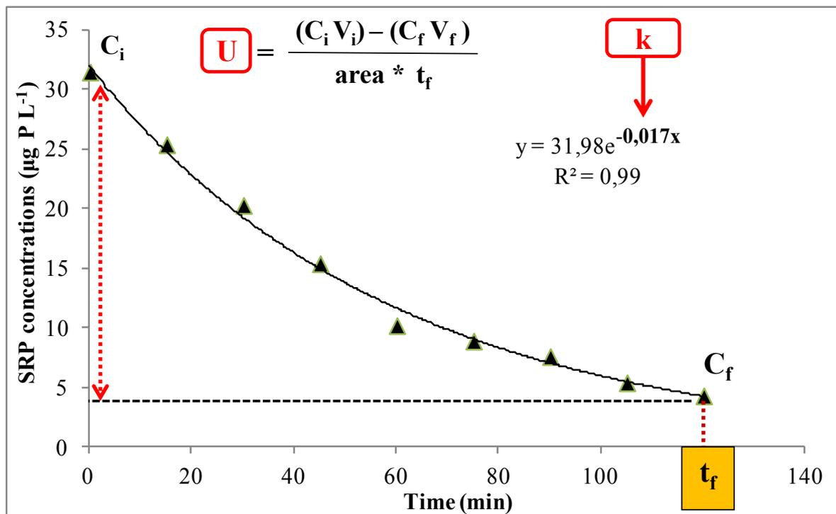
**Figure 1.** Example of dissolved inorganic phosphorus decay in time after controlled spike in response to biotic uptake by river biofilms. Uptake rate coefficient ( $K$ ,  $\text{min}^{-1}$ ) is calculated by fitting negative exponential curve to the data. The phosphate uptake rate ( $U$ ) was calculated as the mass of phosphorous removed from the water column per unit area per unit time ( $\mu\text{g P cm}^{-2} \text{min}^{-1}$ ).
