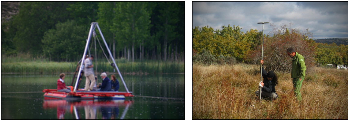
Fig. 34. On the left, the floating raft platform equipped with a piston corer at Somolinos lake. On the right, russian corer sampling a peat bog in northern Guadalajara.
