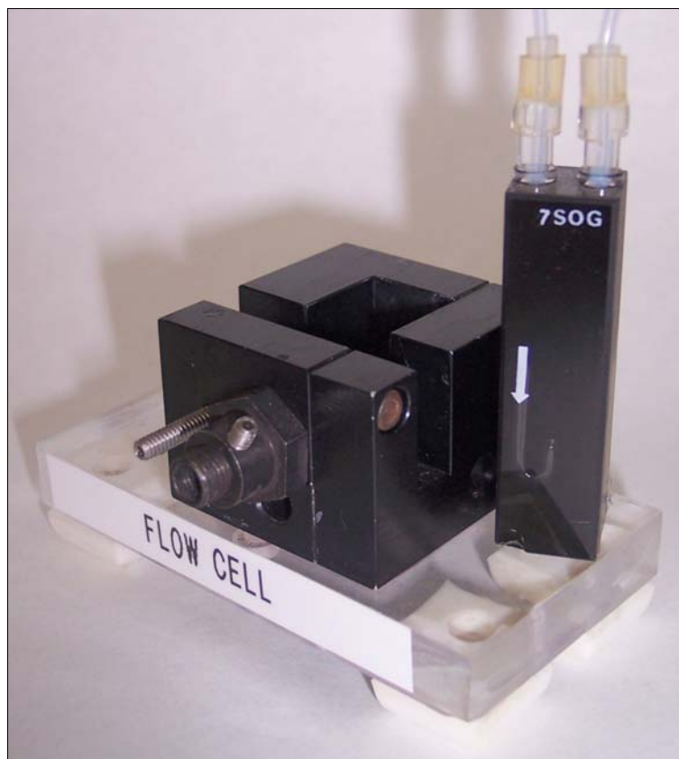
Figure 12: Cuvette holder CUV-UV with connections for fiber optics and special optical glass flow cell (1 cm, 14 \mu l dead volume).
