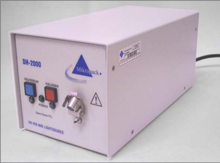
Figure 14: Light source DH-2000-DUV with front side connection for the optical fiber (open safety lid) and power buttons for halogen and deuterium bulbs.
