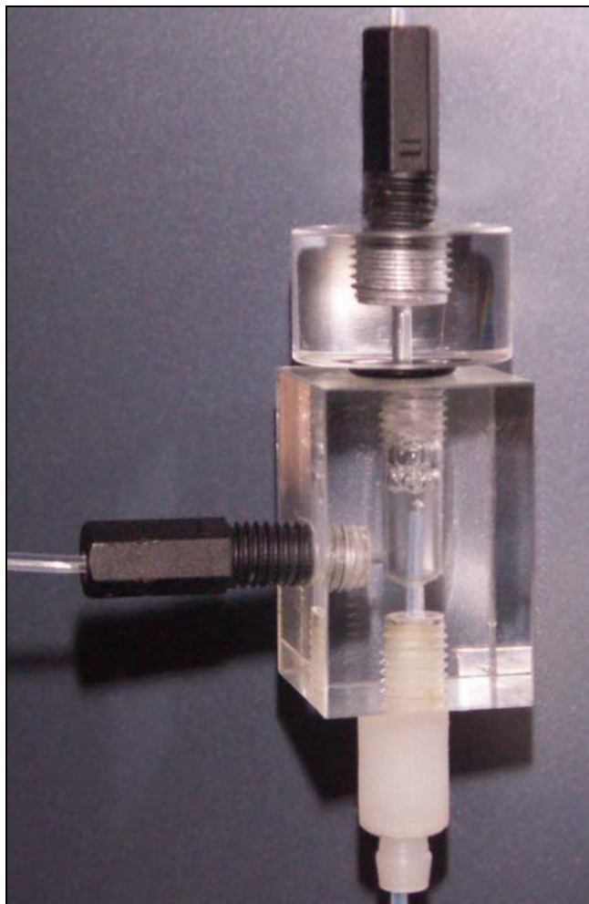
Figure 10: Bubble separator to be used in the sample transport line for monitoring. Bubbles entering from below keep stacked in the head space of the cell and are drawn off from time to time by an additional pump. The sample stream flows out on the left side.
