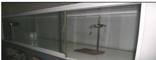
Figure 9: Wind tunnel used on insect behavioral assays.
