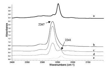
**Figure 9.** FT-IR spectra of PrN in CCl<sub>4</sub> solution (a), NaMOR in the presence of PrN vapors (b) and after evacuation at room temperature (c), 373 K (d) and 473 K (e).
