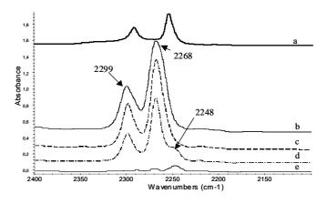
Figure 7. FT-IR spectra of AN in CCl<sub>4</sub> solution (a), NaMOR in the presence of AN vapors (b) and after evacuation at room temperature (c), 373 K (d) and 473 K(e).
