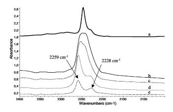
**Figure 7.** FT-IR spectra of IBN in CCl<sub>4</sub> solution (a), NaX in the presence of IBN vapors after evacuation at room temperature (b), at 373 K (c), 423 K(d) and 473 K (e).
