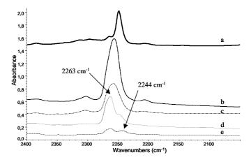
**Figure 5.** FT-IR spectra of PrN in CCl<sub>4</sub> solution (a), NaY in the presence of PrN vapors after evacuation at room temperature (b), at 373 K (c), 423 K(d) and 473 K (e).
