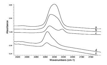
**Figure 13.** FT-IR of adsorbed PN on NaX evacuated at room temperature (a), at 373 K (b) and 473 K (c), and on NaSilicaAlumina evacuated at room temperature (d), and at 373 K (e).
