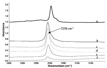
**Figure 9.** FT-IR spectra of IBN in CCl<sub>4</sub> solution (a), NaY in the presence of IBN vapors after evacuation at room temperature (b), at 373 K (c), 423 K(d), 473 K (e) and 523 (f).
