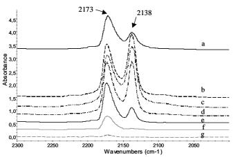
**Figure 5.** FT-IR spectra of HMOR in the presence of CO gas taken immediately at 133 K (a) and after 2 min (b), and under evacuation at 133 K (c), 143 K (d), 173 K (e), 193 (f) and 213K (g) on the CO stretching range.
