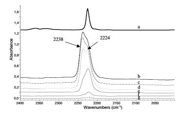
**Figure 14.** FT-IR spectra of liquid oTN (a), KMOR in the presence of oTN (b) and after evacaution at room temperature(c) at 473 K (d), at 573 K (e), at 673 K (f) and at 773 K (g).
