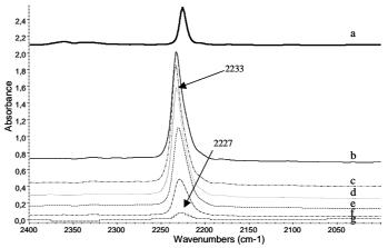
**Figure 15.** FT-IR spectra of liquid oTN (a), CsMOR in the presence of oTN (b) and after evacaution at room temperature(c) at 473 K (d), at 573 K (e), at 673 K (f) and at 773 K (g).
