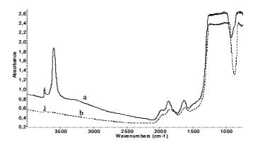
**Figure 3.** FT-IR spectra of activated HMOR (a) and NaMOR (b) samples at 773 K in vacuum conditions.
