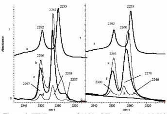
**Figure 3.** FT-IR spectra of AN in CCl<sub>4</sub> solution (a), NaX in the presence of AN vapors after evacuation at 373 K (b), 423 K(c) and 473 K (d), NaY in the presence of AN vapors after evacuation at 300 K (e), 373 K (f) and 423 K(g).
