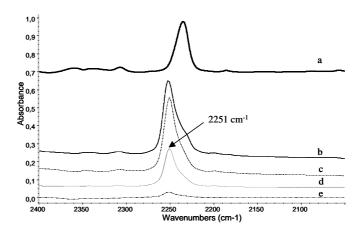
**Figure 10.** FT-IR spectra of PN in CCl<sub>4</sub> solution (a), NaY in the presence of PN vapors after evacuation at room temperature (b), at 373 K (c), 423 K(d) and 473 K (e).
