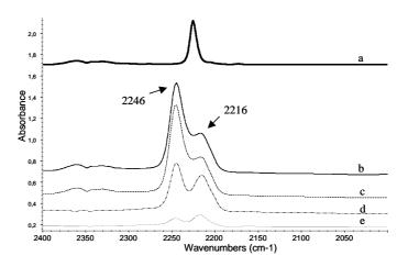
**Figure 13.** FT-IR spectra of liquid oTN (a), in the presence of oTN (b) and after evacaution at room (c) at 473 K (d) and 573 K (e).
