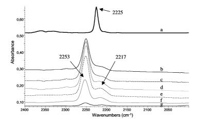
**Figure 12.** FT-IR spectra of liquid oTN (a), LiMOR in the presence of oTN (b) and after evacaution at room temperature(c) at 473 K (d), 573 K (e), 673 K (f) and 773 K (g).
