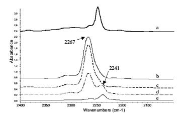
**Figure 8.** FT-IR spectra of PrN in CCl<sub>4</sub> solution (a), NaMOR in the presence of PrN vapors (b) and after evacuation at room temperature (c), 373 K (d) and 473 K (e).
