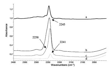
**Figure 10.** FT-IR spectra of liquid PrN (a), KMOR in the presence of PrN after evacaution at room temperature (b) at 373 K (c) and 473 K (d).
