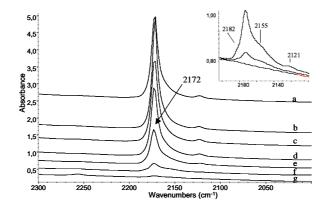
**Figure 2.** FT-IR spectra of activated NaY in the presence of CO gas under evacuation at 133K (a), 143K (b), 153 K (c), 163 K (d), 173 (e), 193 K (f) and 203 (g) in the CO stretching range.
