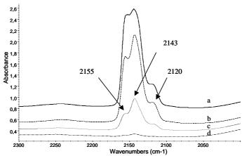
**Figure 7.** FT-IR spectra of CsMOR in the presence of CO under evacuation at 133 K (a), at 143 K (b), 153 K (c), 163 K (d), 173 K (e), 183 K (f) and 193 K (g) on the CO stretching range.
