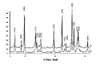
Figure 1. X-ray Diffraction patterns of NaMOR (a) and HMOR (b) samples.
