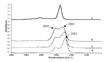
Figure 10. FT-IR spectra of PN in CCl<sub>4</sub> solution (a), NaMOR after evacuation at room (b), at 373 K (c) and 473 K (d).
