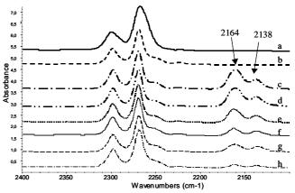
**Figure 14.** FT-IR of adsorbed AN on NaMOR at room temperature (a) evacuated at 373 K and cooled at 133 K (b) after CO adsorption at 133K (c), under evacuation at 143 K (d), 173 K (e), 193 K (f), 213 K (g), 233 K (h).
