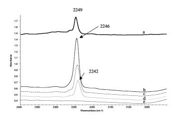
**Figure 11.** FT-IR spectra of liquid PrN (a), CsMOR in the presence of PrN after evacuation at room temperature (b) at 373 K (c), 473 K (d) and 573 K (e).
