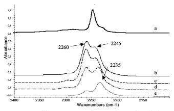
**Figure 9.** FT-IR spectra of IBN in  $CCl_4$  solution (a), NaMOR in the presence of IBN vapor (b) and after evacuation at room temperature (c), 373 K (d) and 473 K (e).
