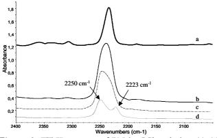
**Figure 8.** FT-IR spectra of PN in CCl<sub>4</sub> solution (a), NaX in the presence of PN vapors after evacuation at room temperature (b), at 373 K (c), and 473 K (d).
