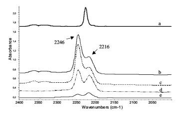
**Figure 12.** FT-IR spectra of liquid oTN (a), in the presence of oTN (b) and after evacaution at room (c) at 473 K (d) and 573 K (e).
