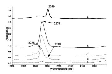
**Figure 8.** FT-IR spectra of liquid PrN (a), LiMOR in the presence of PrN after evacaution at room temperature (b) at 373 K (c), 473 K (d) and 573 K (e).
