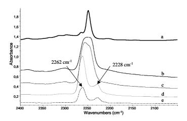
**Figure 4.** FT-IR spectra of PrN in CCl<sub>4</sub> solution (a), NaX in the presence of PrN vapors after evacuation at room temperature (b), at 373 K (c), 423 K(d) and 473 K (e).
