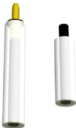
Figure 3.7 – GC home-made electrode coated by a Teflon body.
