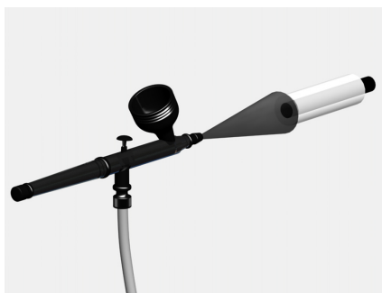
Figure 3.4 – Scheme of deposition of the CNTs by spraying technique onto a glassy carbon substrate.
