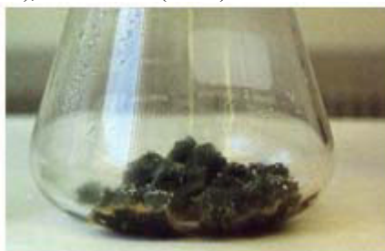
Fig. 2. The white-rot fungus T. hirsuta grown on cubes of nylon sponge (inert support) under SSF conditions
