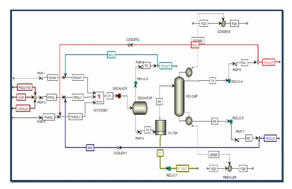
Figure 32. Micro-capsules recuperation process with distillation tower. Block 1 represents the micro-devices
