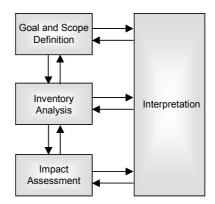
Figure 4. The phases of LCA according to ISO 14040 (2006)
