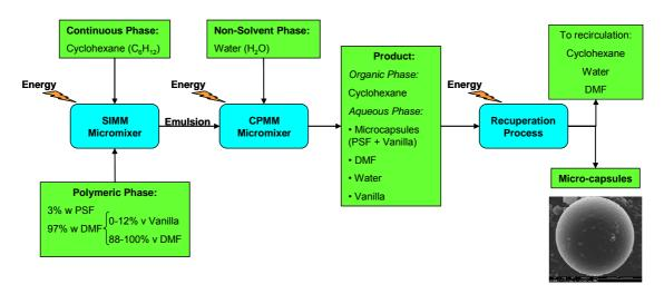
Figure 31. Micro-encapsulation process
