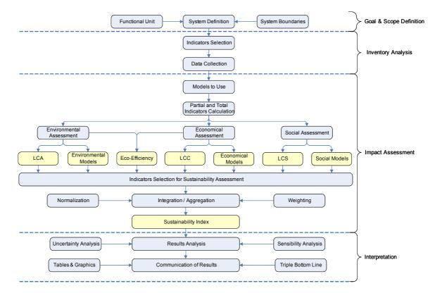
Figure 21. General diagram of the SLCM methodology
