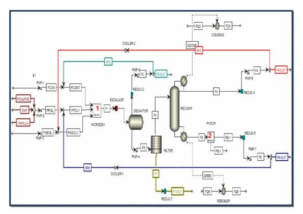
Figure 33. Micro-capsules recuperation process with combined distillationpervaporation. Block 1 represents the micro-devices. Block 2 represents the pervaporation units
