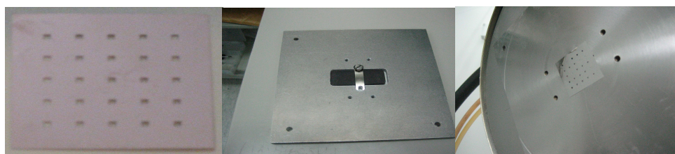
Figure 11: From left to right, shadow mask, back side of the holder showing the magnet used to set in place the shadow mask and front view of the holder with the shadow mask.
