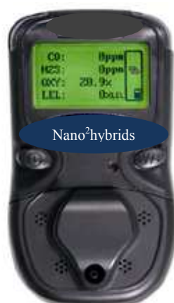
Figure 30: first prototype hand-held unit for selective benzene detection
