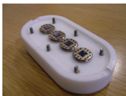
Figure 17: Pictures of the stainless steel and Teflon sensor chamber. Closed (on the left) and with its cover open (on the right). The chamber can house up to 4 sensor array chips packaged in standard TO-8. Each chip consists of 4 micromachined gas sensors
