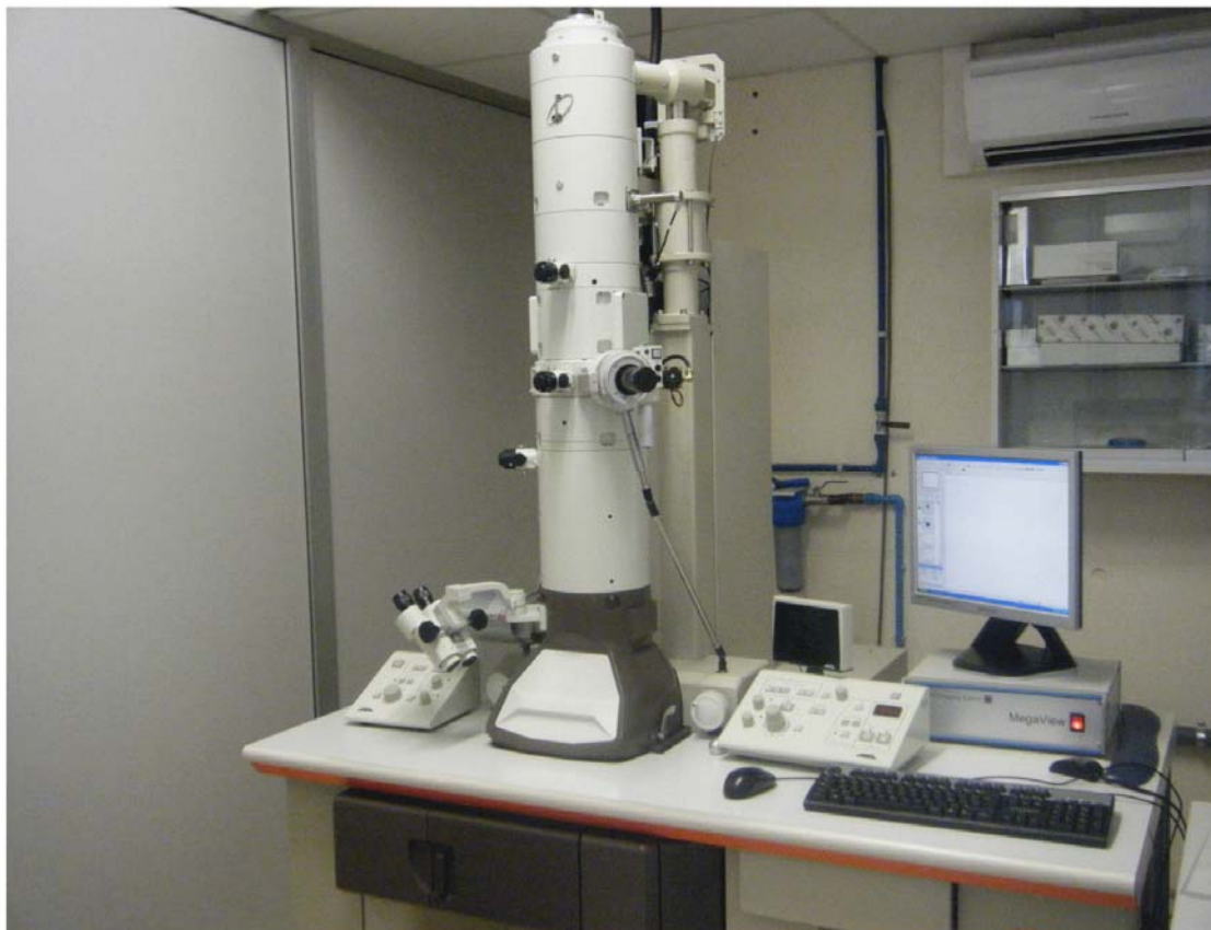
Figure A.2 Transmission electron microscope TEM JEOL 1011 placed at the SRCiT in the URV. Supervised by Mercé Moncusí and Dr. Rita Marimon.
