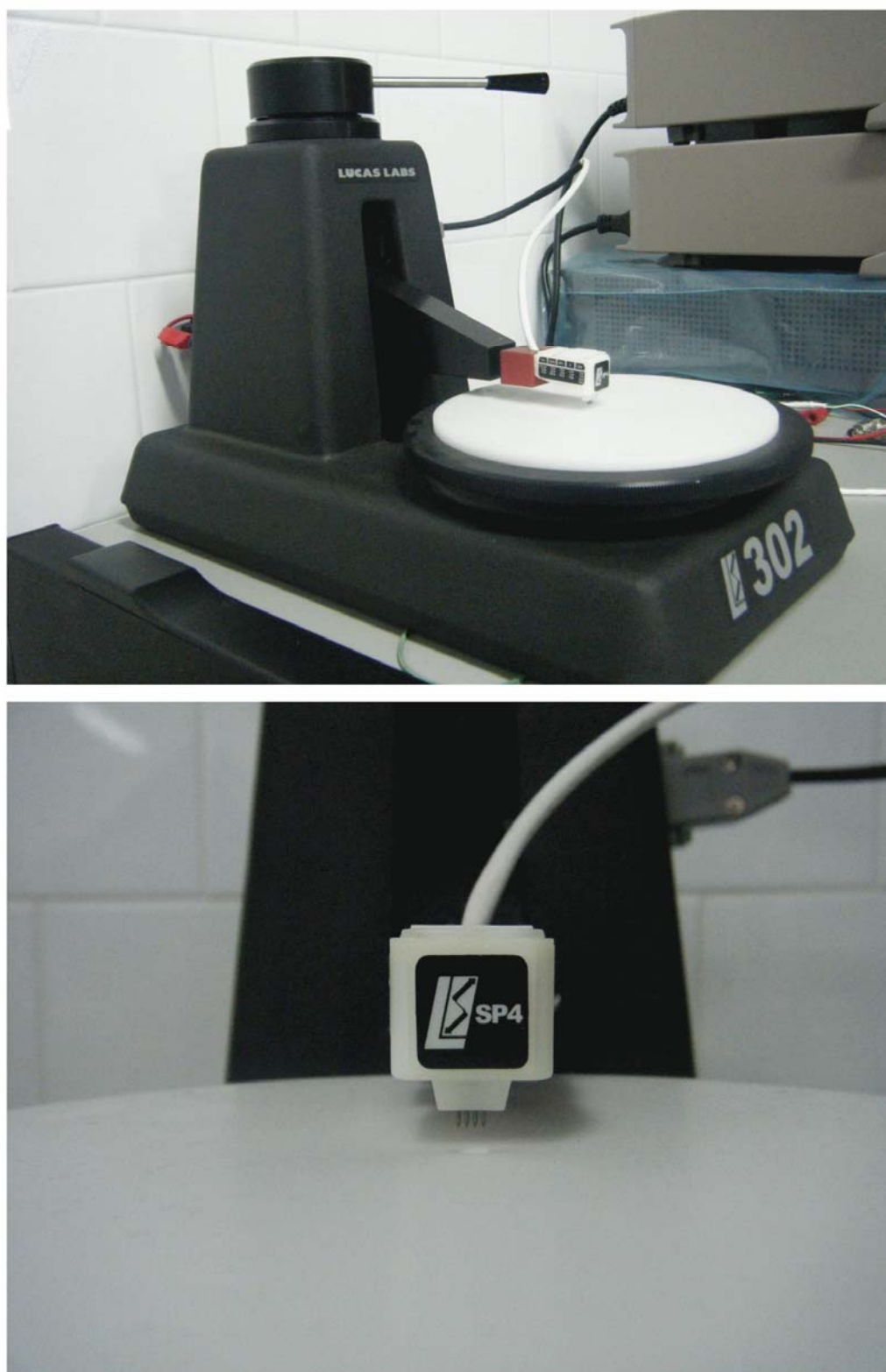
Figure A.5 Four-point probe Lukas Lab located at the optical characterization laboratory in the URV (DEEEiA).
