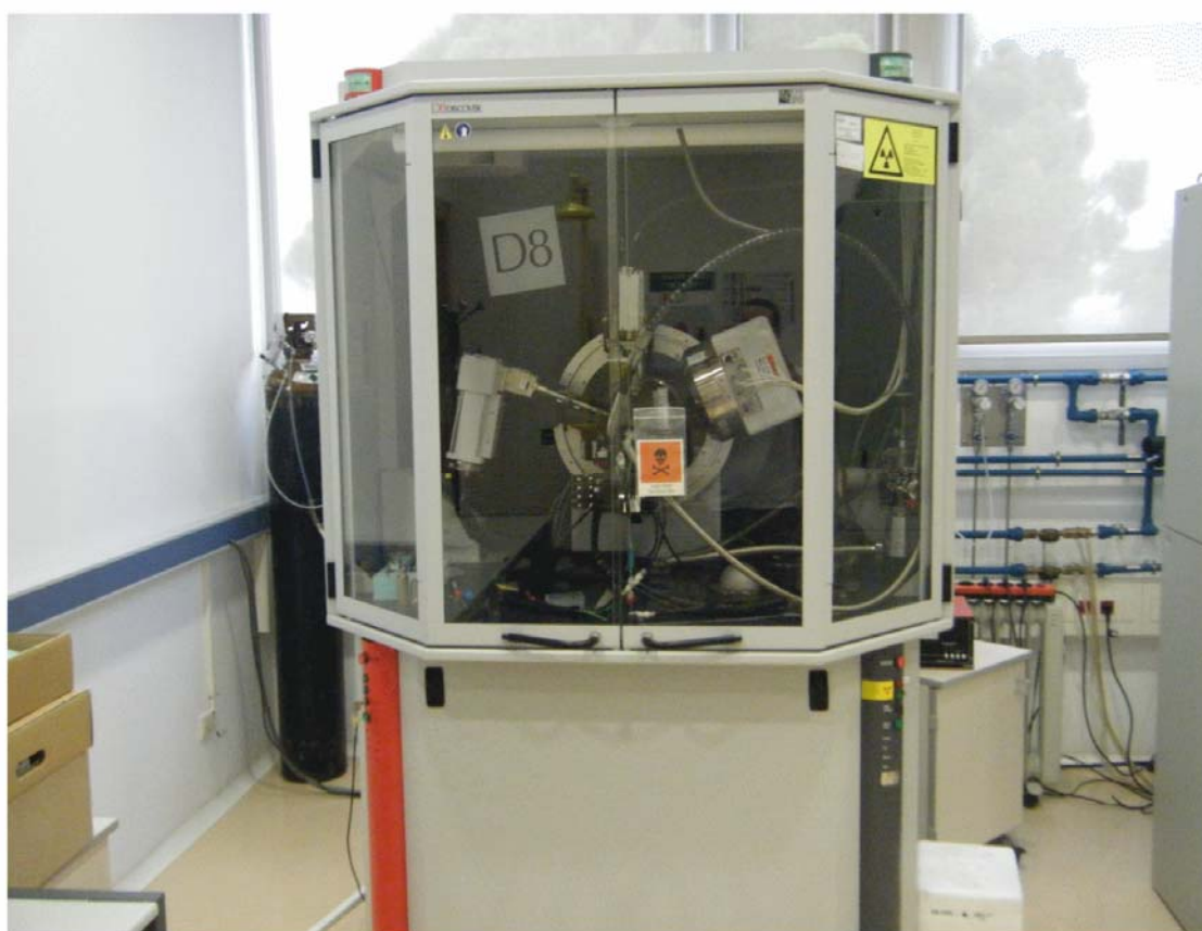
Figure A.4 Micro-X-ray diffractometer Bruker-AXS D8-Discover located at the SRCiT in the URV. Supervised by Dr. Francesc Gispert i Guirado.
