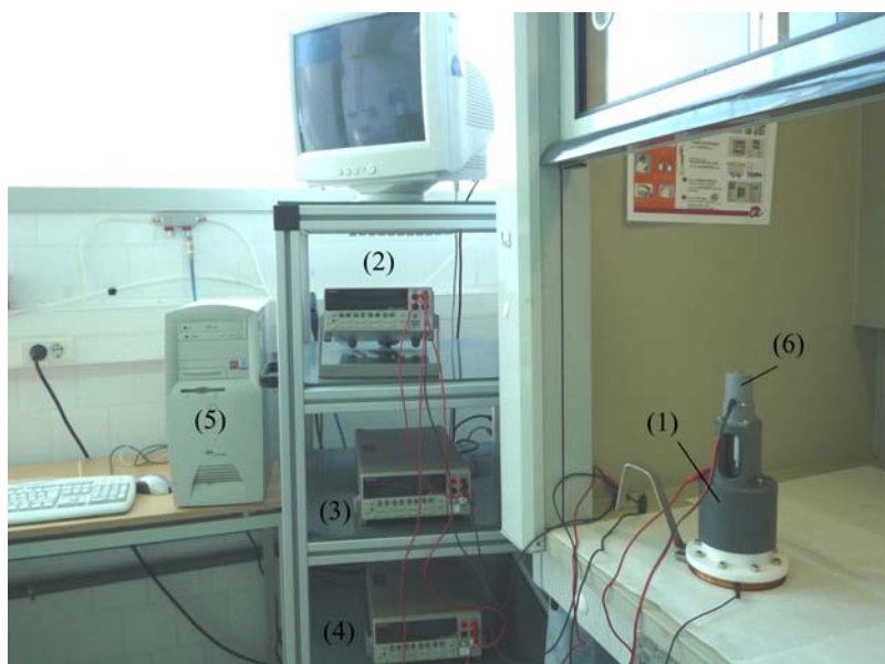
Fig. 3.2. Digital photograph of home-made electrochemical cell and the experimental set-up designed and fabricated for the formation of porous silicon using p-type wafers.
