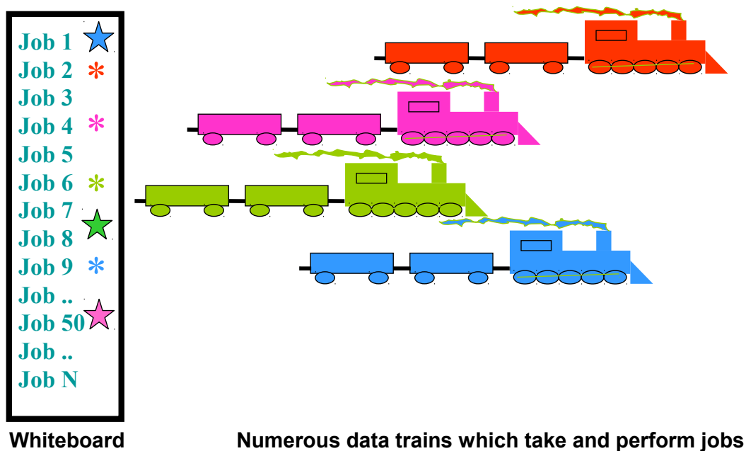
Figure 3.10: A set of Jobs corresponding to sequential sequences of data which cover the entire data range may be posted on a whiteboard. The DataTrain may mark a job as in progress when it starts it and complete when it is finished. When all jobs are done all of the data has been seen once. The whiteboard itself has no special knowledge of the jobs or the overall task - it is a simple mechanism to coordinate potentially hundreds of processes.
