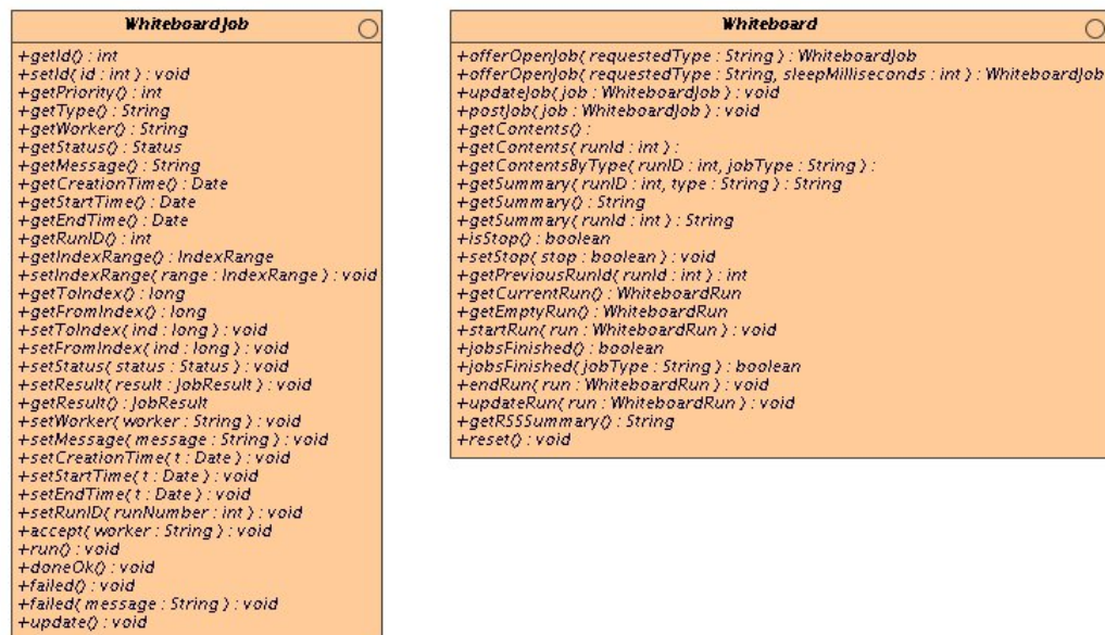
Figure 3.11: The UML interfaces for the Whiteboard and the WhiteboardJob. Note the “postJob” used to populate the whiteboard and “offerOpenJob” methods which the DataTrains use to get jobs. The job itself has methods for status and messages etc.
