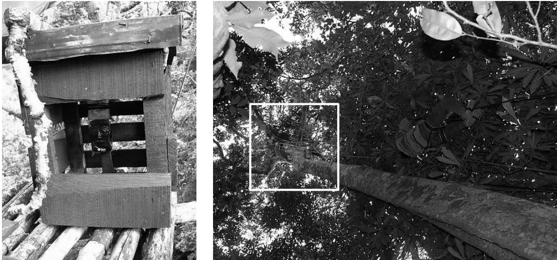
Figure 2.1: Photos of the Canopee project endorsed by Sun Microsystems, India. The first photo shows a box in which one SunSpot is installed. The second photo shows a ground view of a tree on which a sensor is located. Although difficult to appreciate, the red line indicates the presence of one of these container boxes with a sensor inside.
