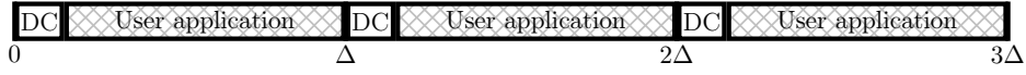
Figure 4.25: Time management between the duty-cycling mechanism and possible user applications. The protocol is organized in a sequence of time periods of length \Delta . The first phase of each period is dedicated to duty-cycling (DC), whereas the second phase is concerned with user applications.
