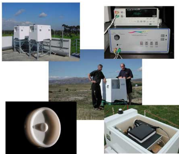
Figure 1.8 Pictures of the NIWA-built spectroradiometer. Top left: Two NIWA systems. Top right: Power Supply & meter. Centre: NIWA system under test. Bottom left: PTFE Diffuser. Bottom right: Interior of temperature stabilized weatherproof box (source: www.niwa.co.nz).
