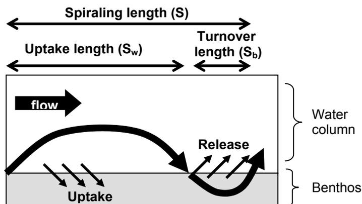
**Figure 3.** Scheme of two-compartment nutrient spiraling model. (Modified from Newbold, 1992).
