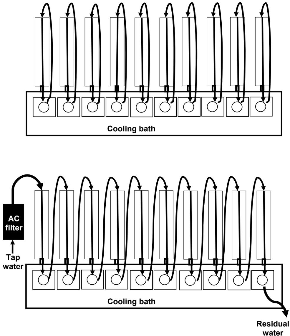
**Figure 1.** Scheme of the experimental channels in recirculating mode used during the colonization of periphyton and short-term Cu toxicity experiment (upper panel) and one-flow through mode used during the Cu and  $\text{PO}_4^{3-}$  retention experiments (lower panel).
