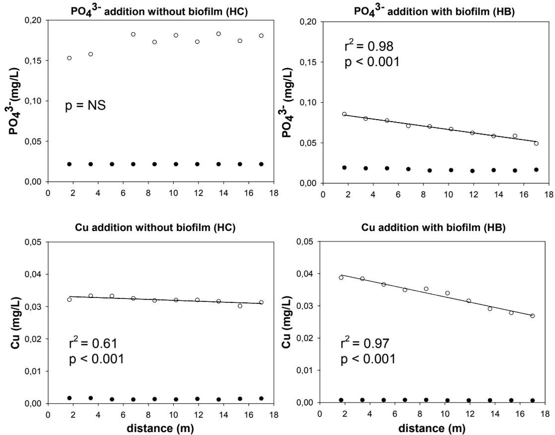
**Figure 3.** Illustrative examples of results from solute additions showing longitudinal variation of Cu and  $\text{PO}_4^{3-}$  concentrations along the channel system at background (solid circles) and plateau (open circles) conditions. Adjust ( $r^2$ ) and significance ( $p$ ) of the linear regression is also indicated.
