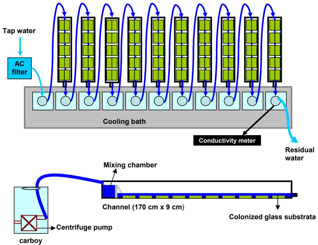
**Figure 1.** Scheme of the experimental channel system showing an aerial view of the water flow connection among channel units (upper panel) and a detailed scheme of the longitudinal section of a channel unit (lower panel).
