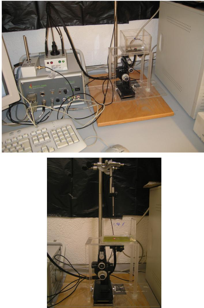
**Figure 1.** Detail of the phyto-PAM chlorophyll fluorometer (upper panel) and measurements on periphyton (lower panel).
