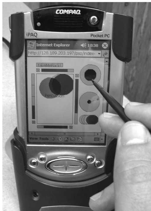
Figure 43. The Public Sound Objects Client Interface running on a PDA
