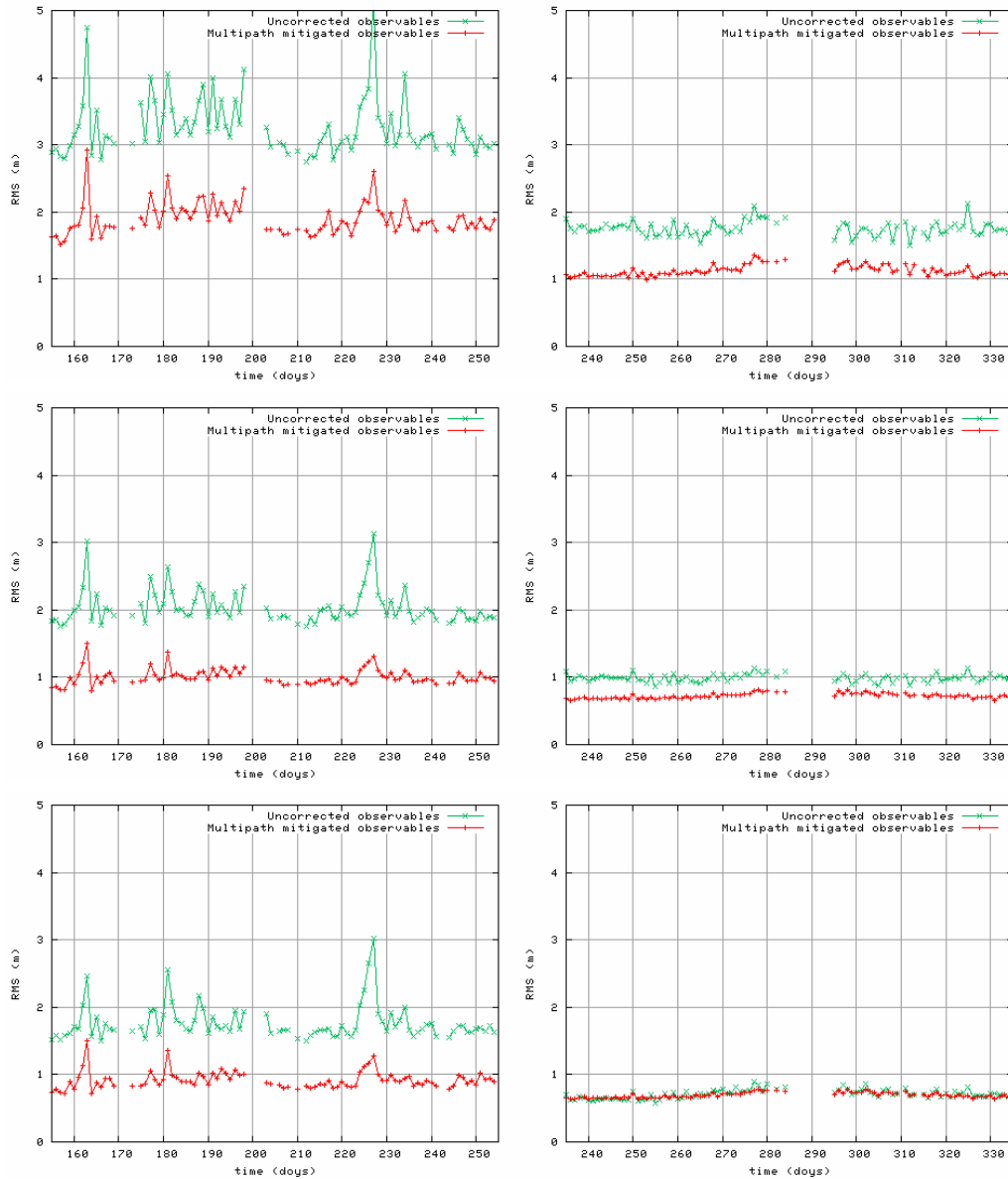
Figure 1.7: Daily 3D positioning error RMS for period a of 100 days in SAC-C (left column, from day 155 to 255) and CHAMP (right column, from day 235 to 335) of 2002. Each point provides the RMS for all the epochs of a single day. First, second and third rows correspond to unsmoothed, 10-sample and 50-sample smoothed observables, respectively.
