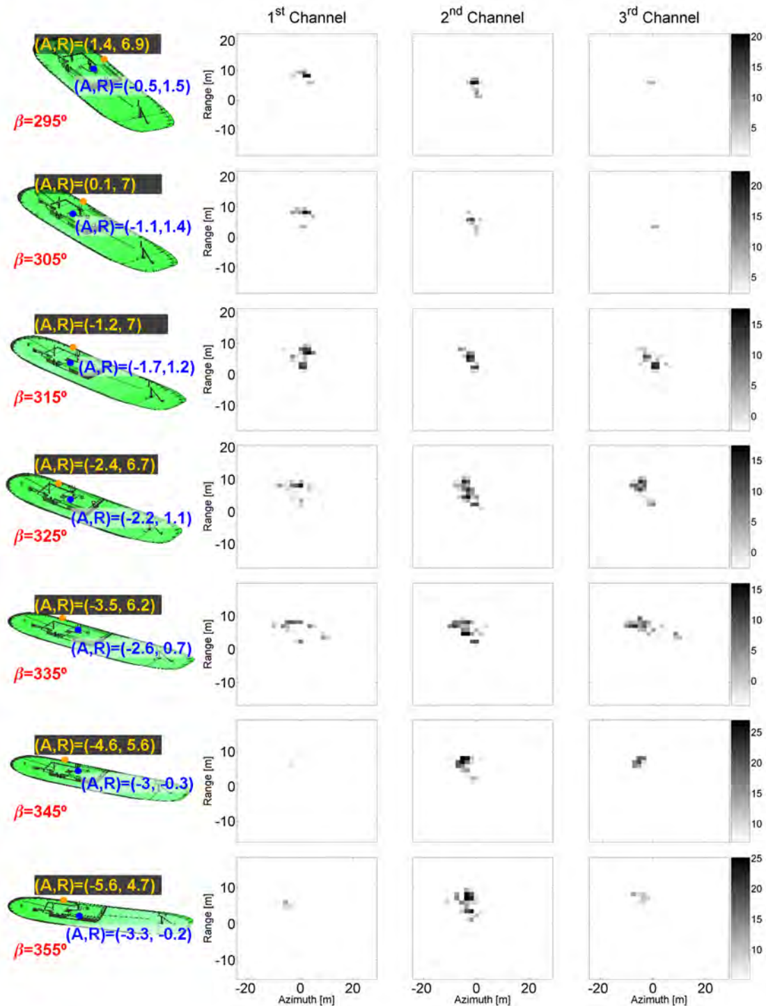
Figure E.20: Weight of the Pauli polarimetric channels related to the polarimetric SAR dataset depicted in Fig. E.19. The values are expressed with respect to the inter-channel maximum value.
