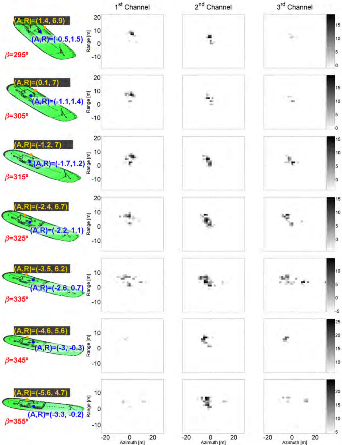
Figure E.8: Weight of the Pauli polarimetric channels related to the polarimetric SAR dataset depicted in Fig. E.7. The values are expressed with respect to the inter-channel maximum value.
