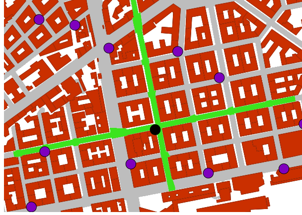
Figure 3.2: Ground coverage \sigma^0 (light green) from a gNB in point p_0 (black) in a portion of the city of Florence. Figure shows also the buildings' shapes s^r (red), the set of points on the street \Lambda (grey) and other gNB locations (purple). © 2022 IEEE
