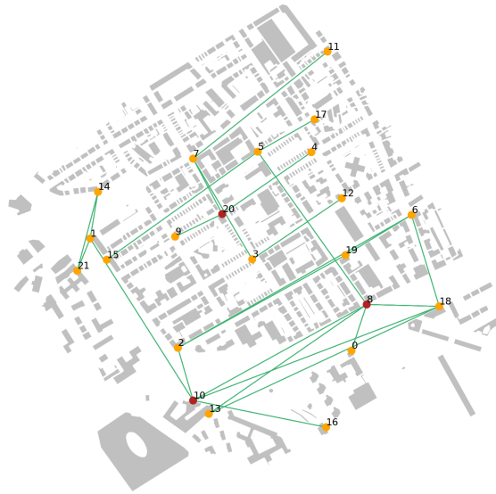
Figure 4.4: Realistic deployment scenario in Florence, Italy. Donors are represented in red, while IAB-Nodes are represented in yellow. © 2023 IEEE
