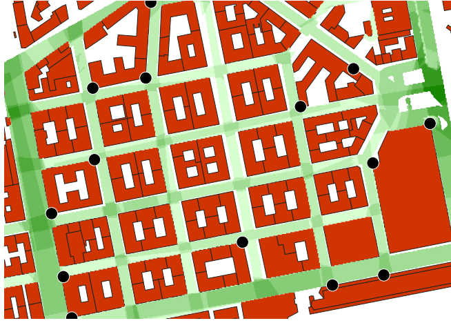
Figure 3.4: Graphical rendering of the coverage \Phi_{[4,45]} (shades of green), and the set of optimal points (black dots) in a portion of one of the considered areas, in Napoli.
