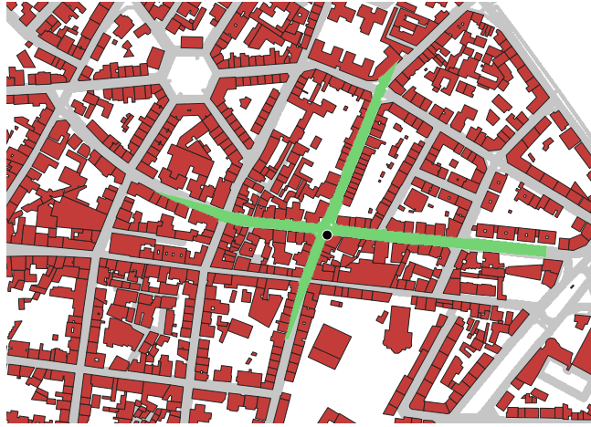
Figure 2.13: Representation of a viewshed computed in an urban area from the corner of a building.
