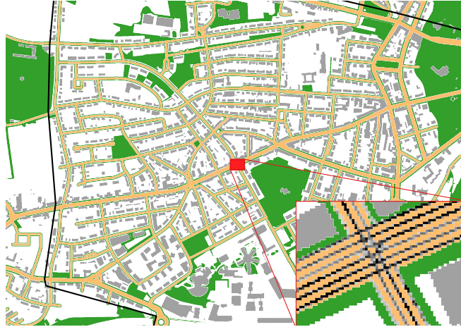
Figure 3.15: Detailed view of a portion of the area considered in the analysis. Yellow highlights roads, green indicates public areas for pedestrians (sidewalks and parks), grey indicates buildings, and white indicates private areas. The zoomed portion shows the vehicular traces with a grayscale representing the number of passages per point (darker means higher).
