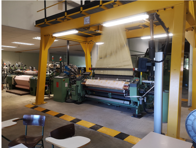
Figure 5.5: Dornier LWV8/J weaving machine moved by a Jacquard Stäubli LX1600B
