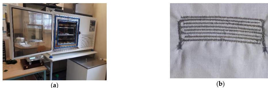
Figure 2. Image of the experimental setup. (a) CCK-25/48 Dycometal (b) Embroidered capacitive sensor.
