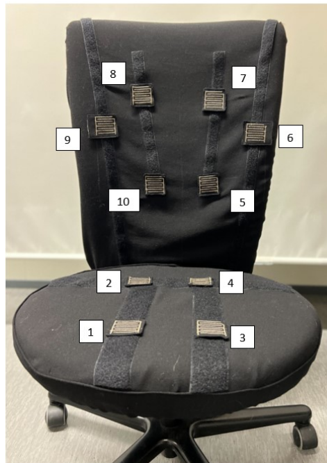
Figure 10.14: Smart chair with sensor distribution and number identification
