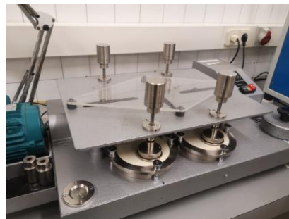
Figure 2. Martindale machine performing a test.
