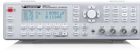
Figure 6.3: Image of the Rohde & Schwarz HM8118 LCR meter used
