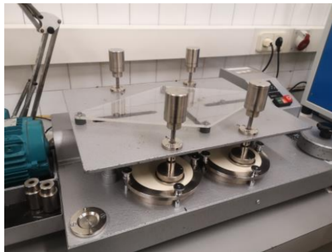
Figure 6.7: Martindale machine performing a test
