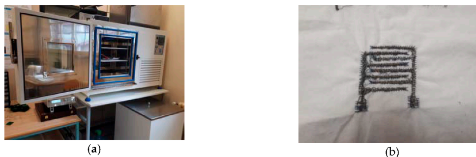
Figure 2. Image of the experimental setup. (a) climatic chamber, (b) embroidered short sensor
