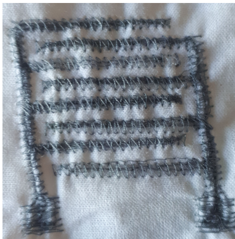
Figure 5.2: Textile capacitive sensor embroidered with satin stitch pattern with a 70% of pattern density.
