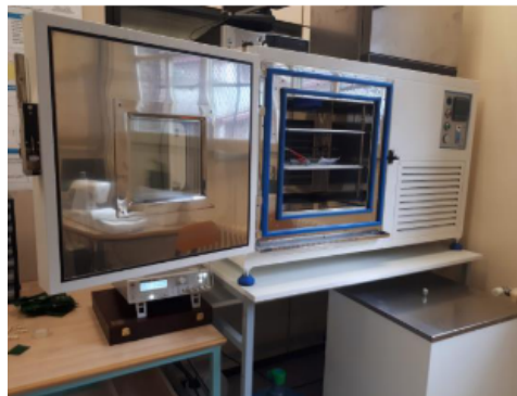
Figure 6.6: Picture of the CCK-25/48 Dycometal climatic chamber used
