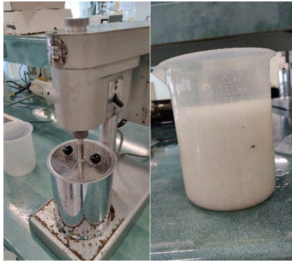
Figure 3.4: Disintegrator (left) and disintegrated Kraft paste (right)
