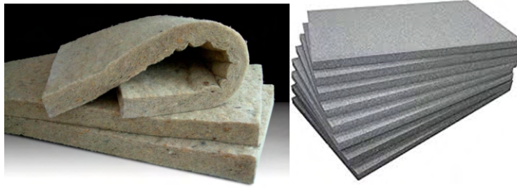
Figure 2.4: Rockwool (left) [46] & EPS (right) [47]
