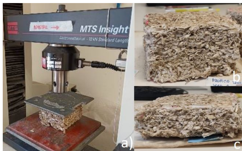
Figure 3.25: a) Compression test b) 40E before test c) 40E after test
