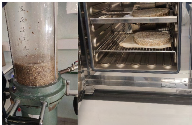
Figure 3.10: Frank sheet former (left) and drying oven (right)
