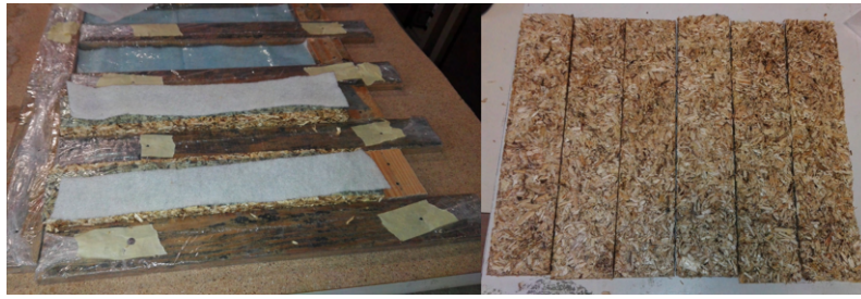
Figure 3.41: Wooden mold with bleeding and absorbent paper (left) and obtained specimens (right)
