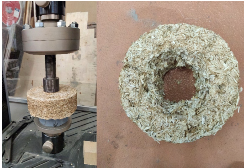
Figure 3.26: Static puncture test - shear test (left) and sample 40E after test (right)
