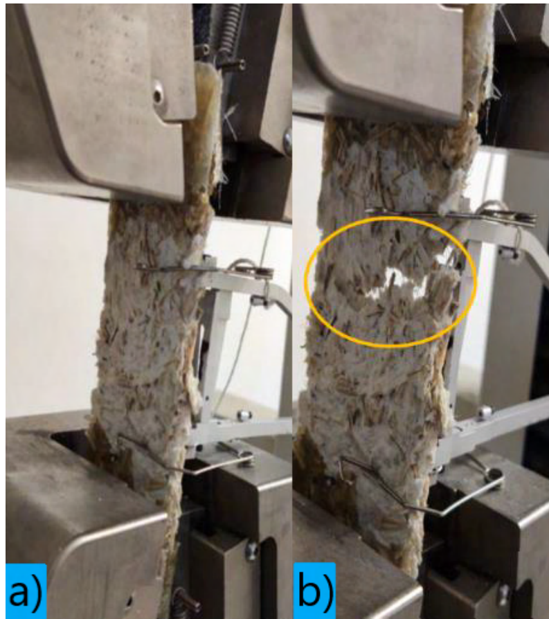
Figure 3.28: a) Tensile test b) ending of the tensile test
