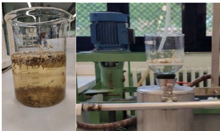
Figure 3.6: Hemp stalk in water (left) and hemp stalk filtered by vacuum (right)
