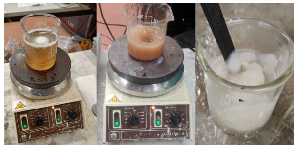
Figure 3.31: Colophony (left), arabic gum (center) and adhesive made with corn starch (right)
