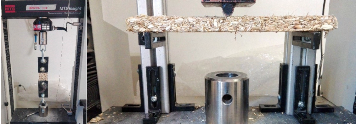
Figure 3.36: Tensile test (left) and bending test (right)
