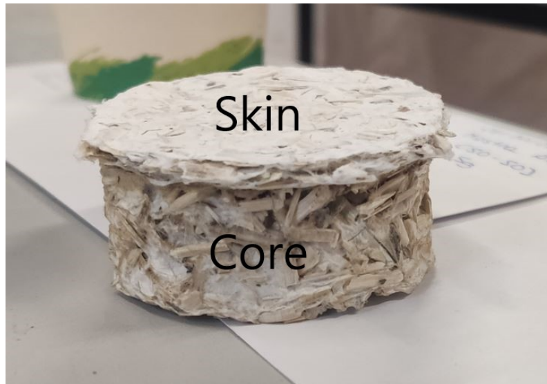
Figure 3.13: Sandwich type sample, core formed with 30E and skin with 50E compressed
