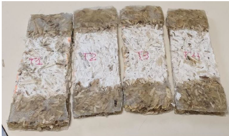
Figure 3.27: Tensile samples with glass fiber to improve the grip
