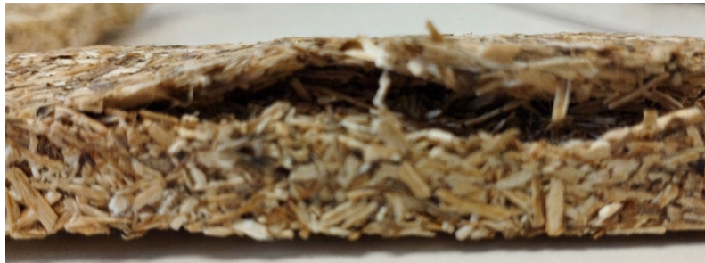
Figure 3.39: Crack formed during drying in the oven at 120°C
