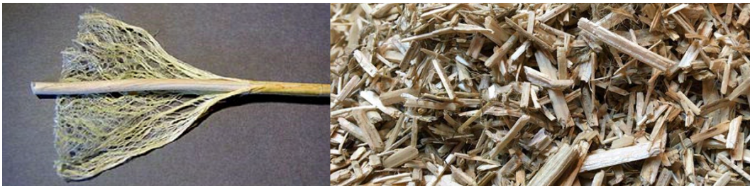
Figure 2.3: Sectioned stem of hemp consisting of plant fibers and hemp stalk [36] & hemp stalk
