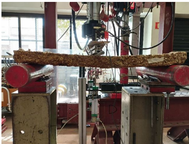
Figure 4.22: Bending test in insulating panels
