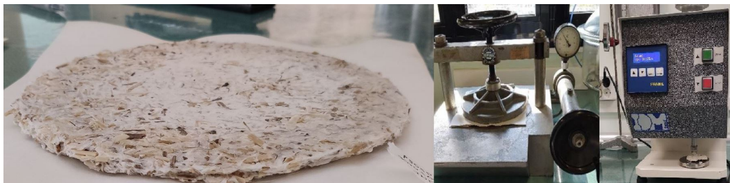
Figure 3.12: Compressed hemp stalk-eucalyptus sample (left), manual paper press (center) and micrometer (right)
