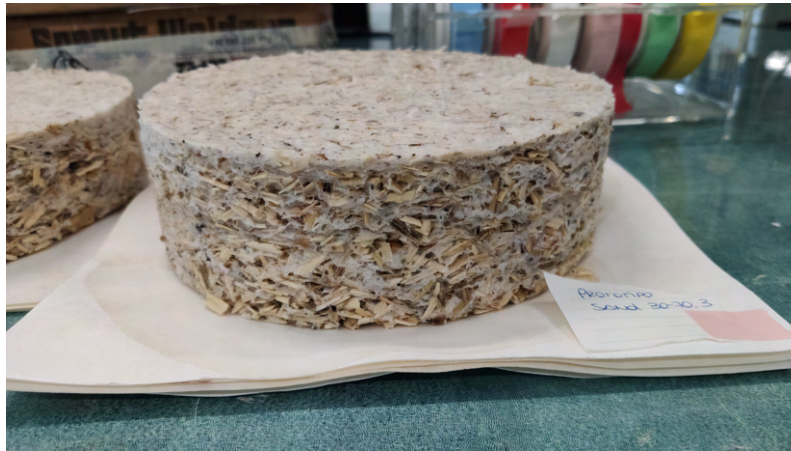
Figure 3.16: Distribution of paper fiber along the sample: top part in the image was in contact with the vacuum
