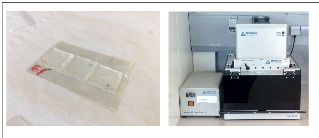
Figure 4.2. Details of the PDMS replica stampers onto the Ormostamp® coated polymeric film, right before UV curing (left), and detail of the UV-curing equipment used (right).
