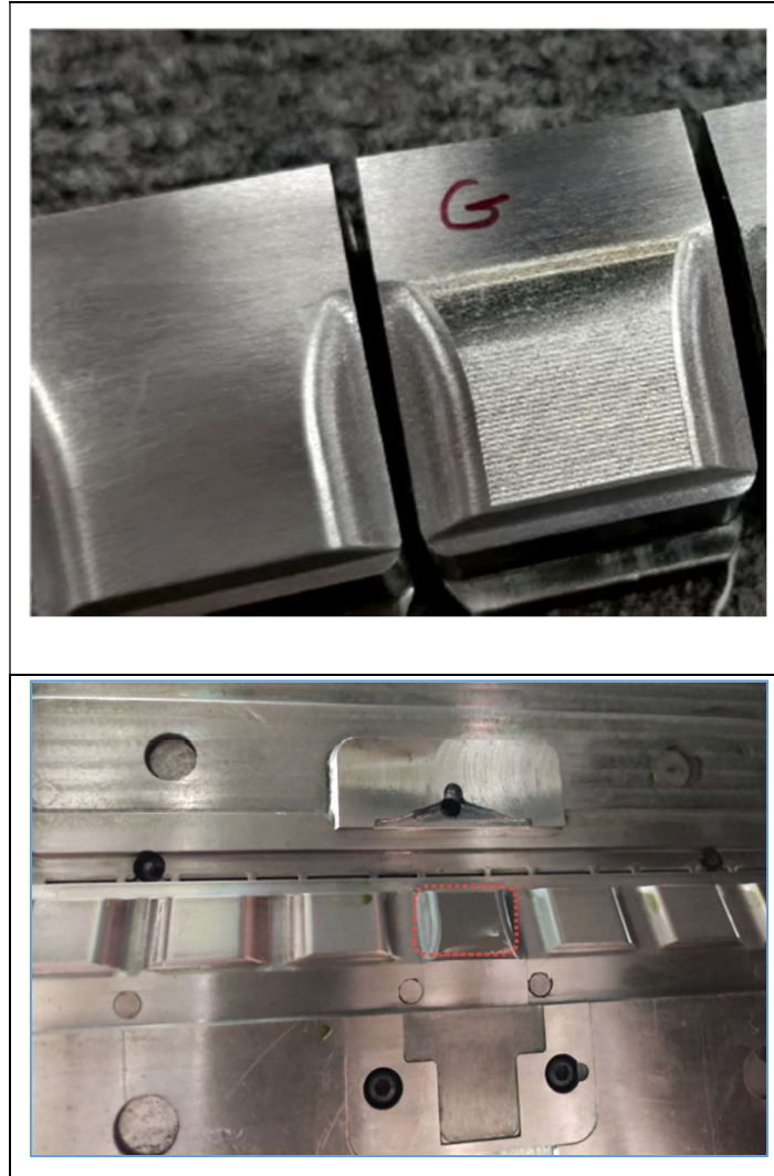
Figure 3.13. Details of the custom-developed microtextured steel insert, shown right next to a nontextured steel insert for comparison (above), and its specific placement on the injection mould cavity (below).
