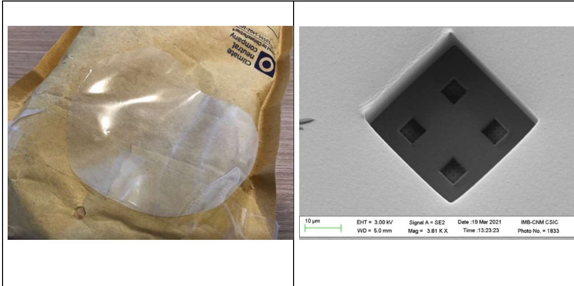
Figure 4.8. Details of the coated and textured film as delivered by ICN2-CNM (left), and 2-level hierarchical negative microstructures present in the replicated Ormostamp® coated films (right). Pictures courtesy of CNM.
