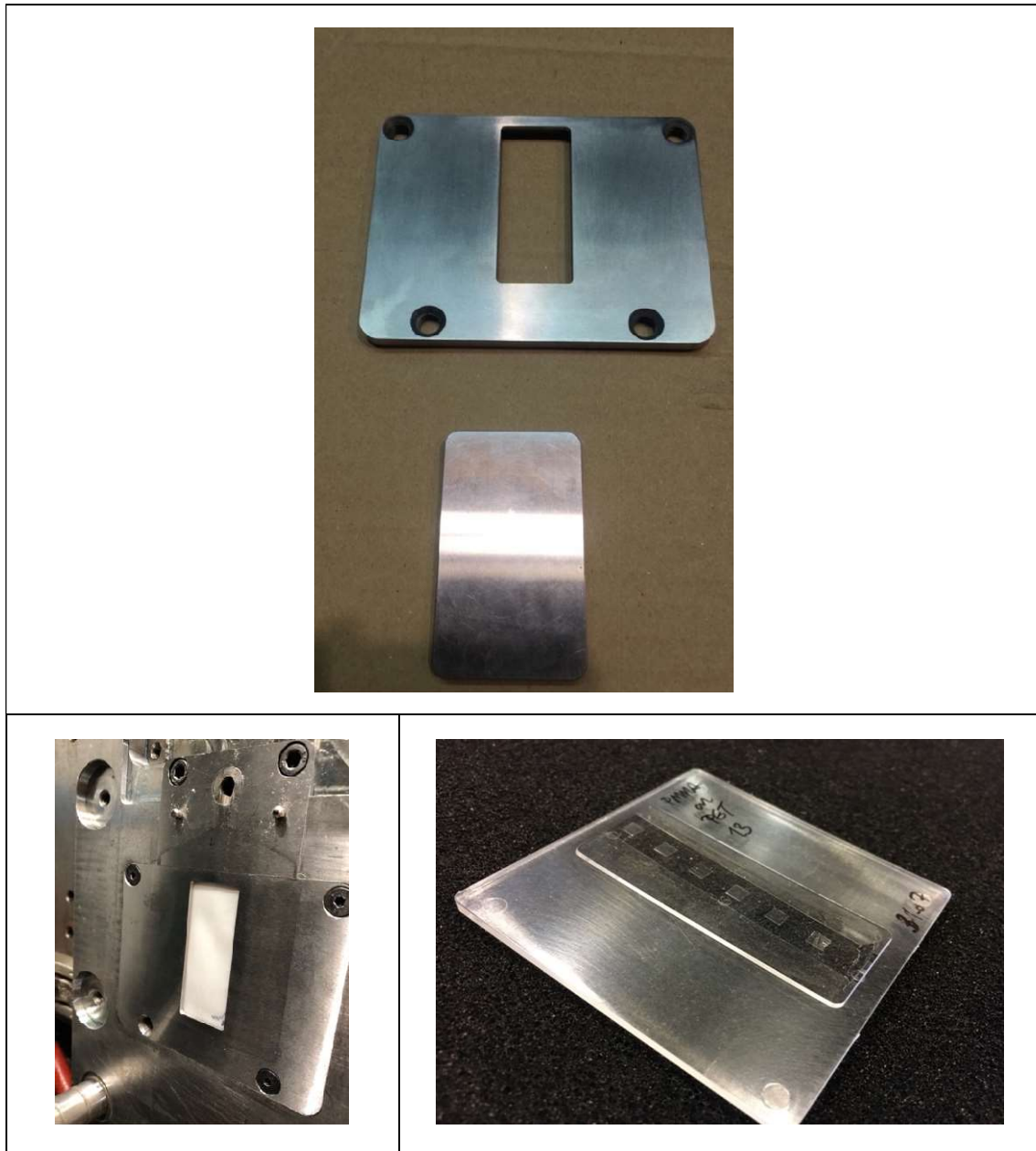
Figure 4.9. Details of the custom designed tool insert for textured film inlay placement during the injection moulding process (above-centre), and actual placement of the steel insert in the injection mould (below-left). Lower-Right image: final part resulting after injection.
