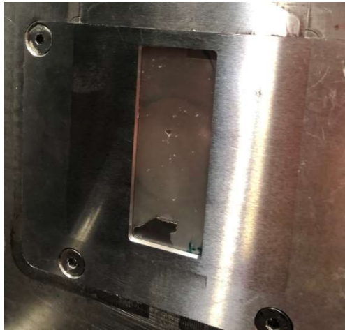
Figure s4.4. Details of the deterioration of the inlay films after various injection shots, showing coating delamination at its lower section.
