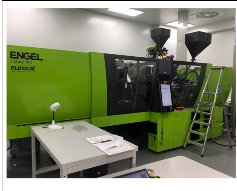
Figure 3.3. Picture of the Engel 3K injection moulding machine used in the experiments. Image credit: EURECAT
