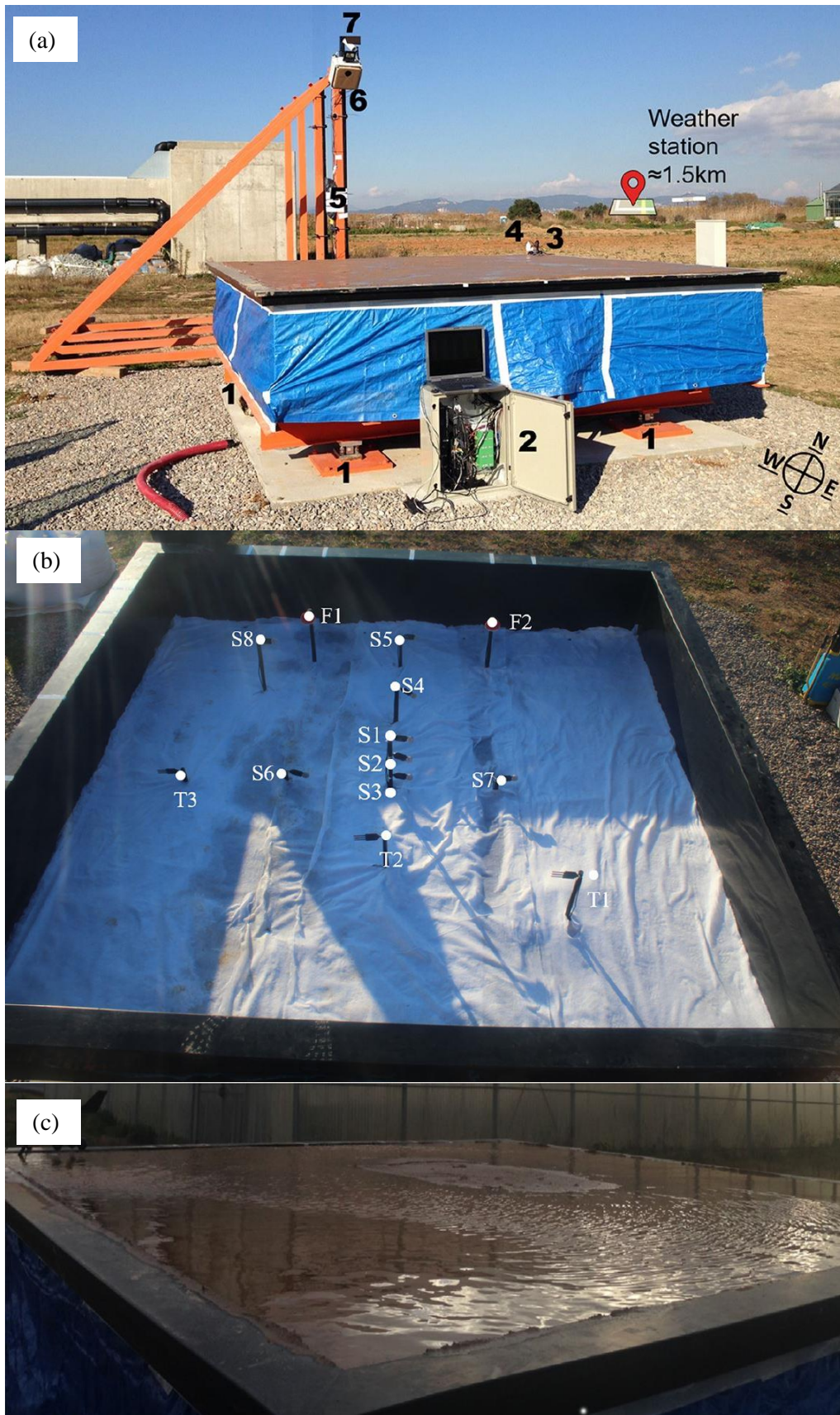
Figure 6-4. Field experiment: (a) setup at the Agròpolis site, (b) empty tray with different embedded sensors locations, and (c) filled tray showing thin water film forming at the surface (Cordero et al., 2021).
