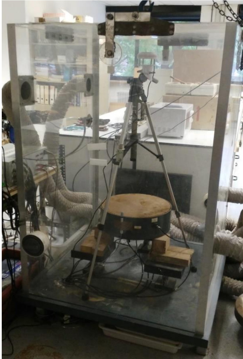
Figure 5-3. Anemometer mounted inside the environmental chamber for wind measurements under test conditions similar to the original.
