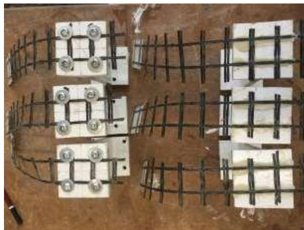
Figure 39. Specimens with mechanical connection (left) and adhesive connection (right)
