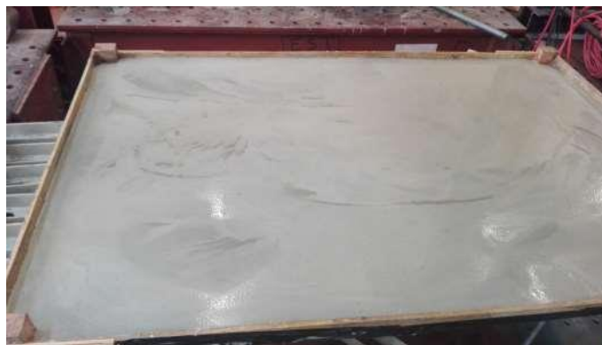
Mortar in curing phase
