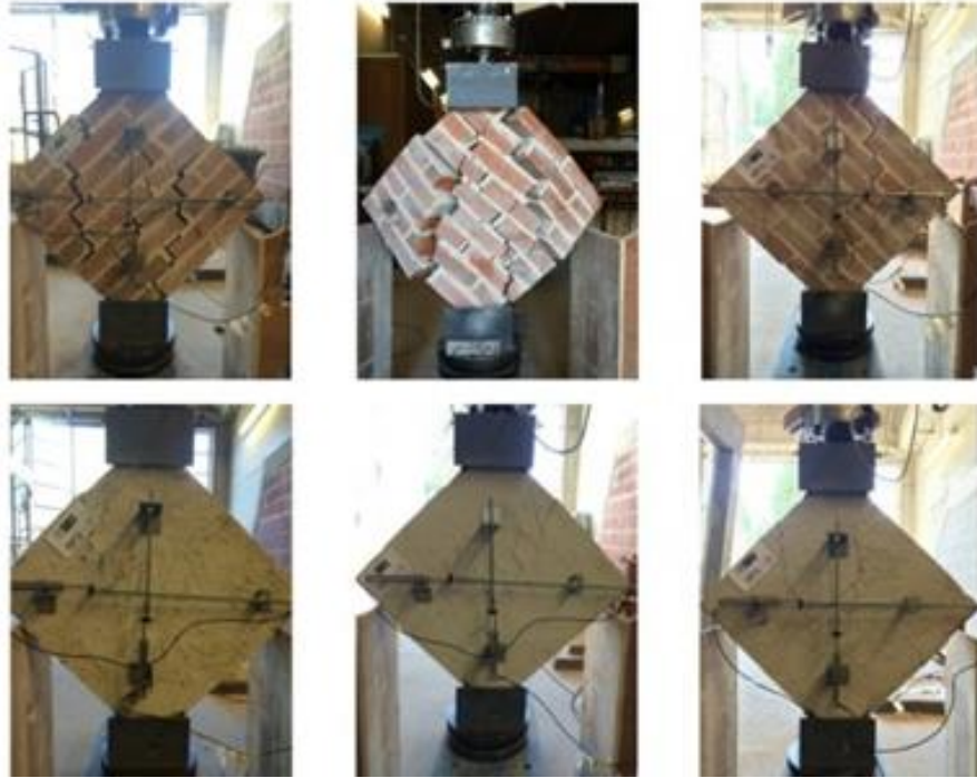
Figure 10. Failure mode of the specimens (Casacci et al. , 2019)
