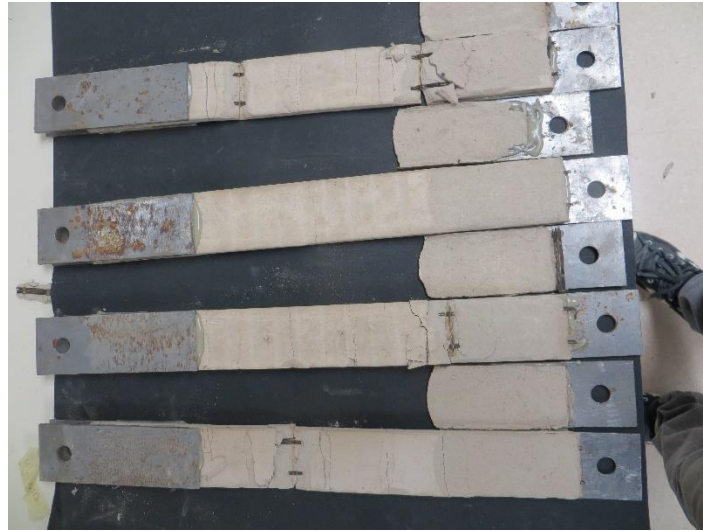
Figure 67. Mesh-mortar connection tests
