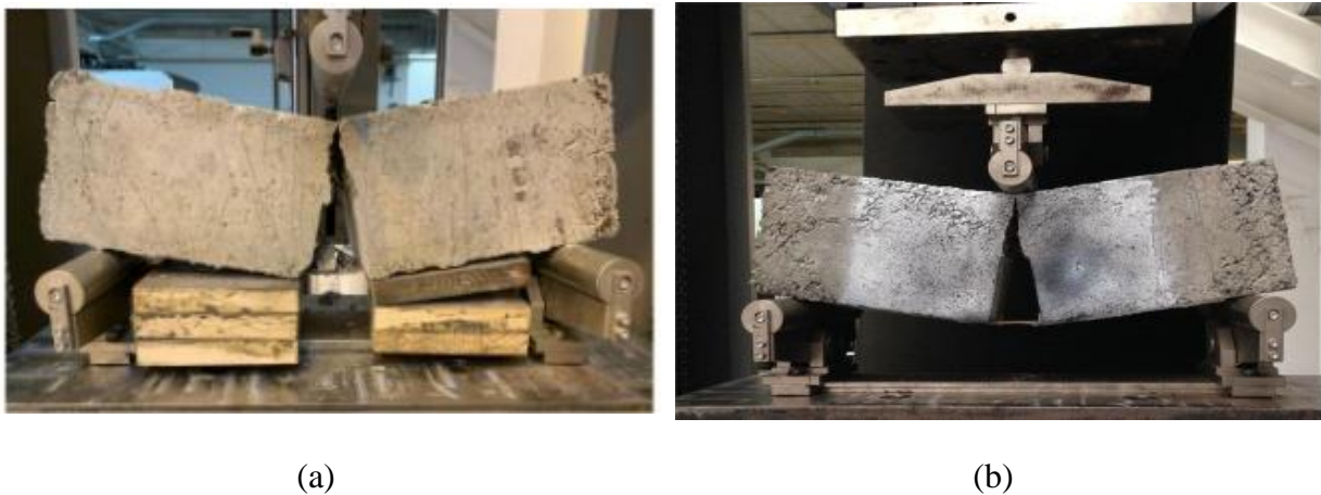
Figure 12. Typical failure mode of (a)CFRP and (b) PBO-FRCM strengthened beams (De Domenico et al. , 2020)
