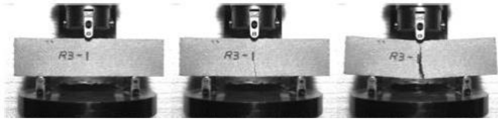
Figure 22. Cracking process of a mortar specimen under flexural test
