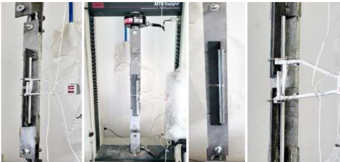
Figure 44. Tensile test setup configuration
