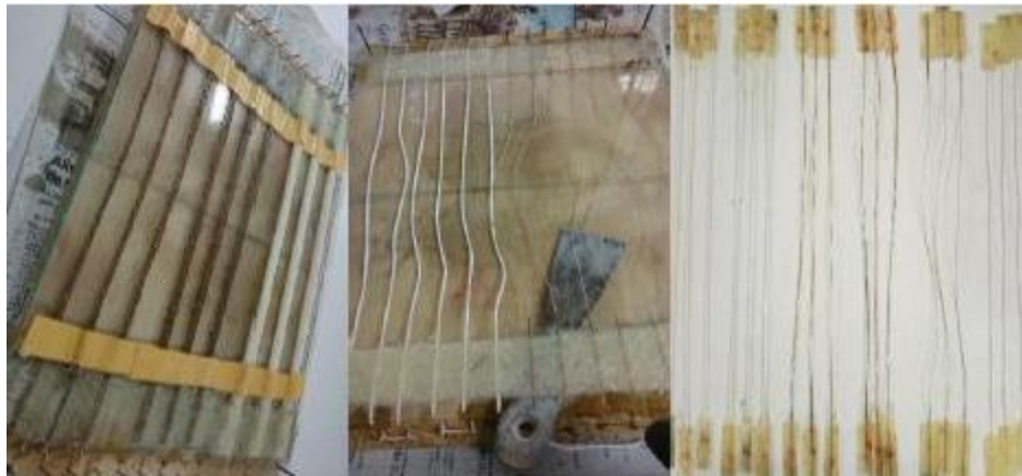
Figure 28. Preparation of yarn and tuft specimens for tensile testing
