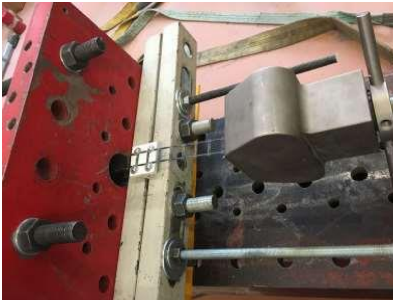
Figure 40. GFRP-mesh test configuration
