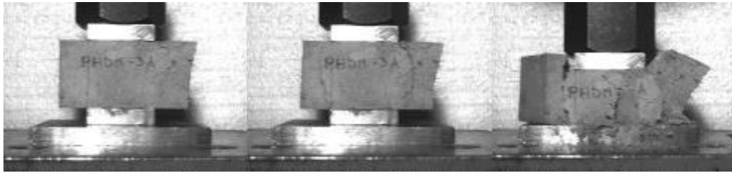
Figure 24. Crushing process of a mortar specimen under compression test
