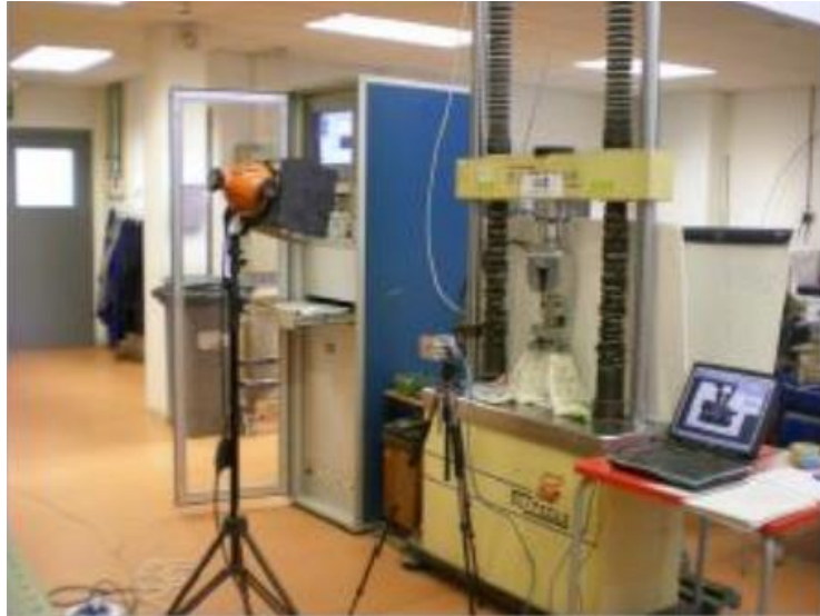
Figure 21. Test setup configuration for mortar characterization
