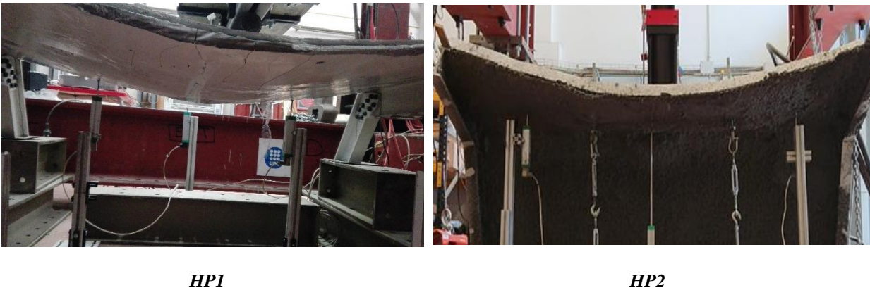
Figure 57. Failure modes in the tests
