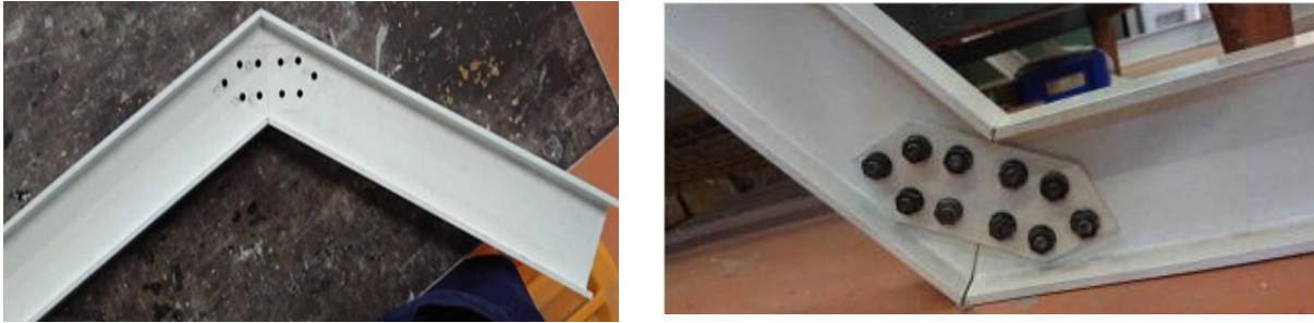
Figure 52. GFRP rib joint for HP2
