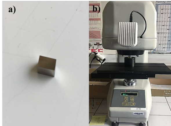
Figure 2.11: Cut and polished sample a), Zwick/Roell Micro Hardness Tester b).
