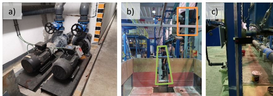
Figure 2.3. (a) Pumping system in the downstream deposit, (b) experimental device looking upstream from the bottom of the spillway tank (black tank in orange and flume in green), and (c) flume's slope measuring tape.
