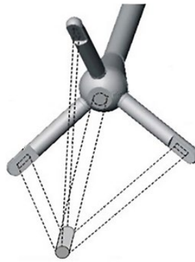
Figure 3.2. Details of a three-beam downward-looking ADV (Source: www.sontek.com ).
