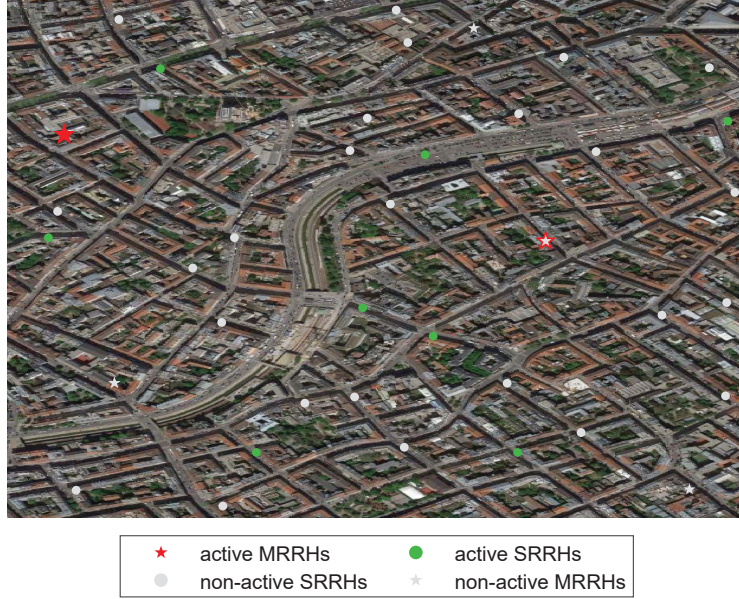
Figure 6.12: Resulting radio network for a C-RAN at 28 GHz with \omega_1 = 0.6 and LT profile.
