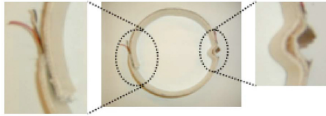
Figure 2.13: IW failure mechanism. Adapted from [52].
