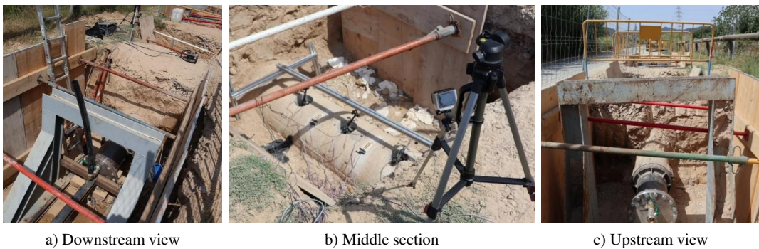
Figure 5.4: Field view of the experimental setup and testing environment during the full-scale on-site test: downstream view (a), middle section of the tested pipe showing severe damage (b) and upstream view (c).
