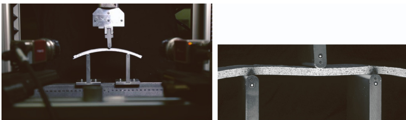
Fig. 10. Digital Image Correlation setup used during the three-point bending test of curved samples.
