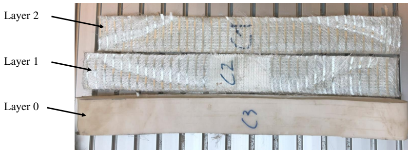
Figure 3.15: Raw liner composition analyzed in the materials verification stage.
