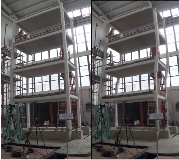
Figure 4: Video frame corresponding to the tests performed on the reinforced concrete frame. The left-hand side corresponds to the original unaltered frame, while on the right, an \times 20 version of the frame shows the operating deflection shape.
