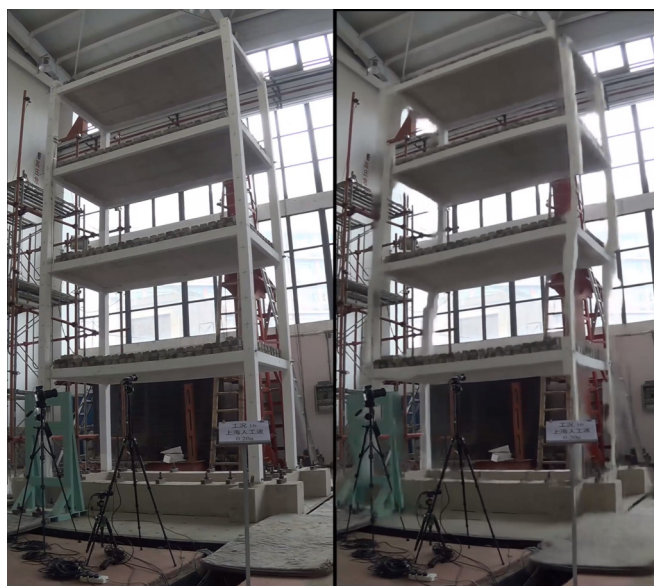
Figure 5.4: Video frame corresponding to the tests performed on the reinforced concrete frame. The left-hand side corresponds to the original unaltered frame, while on the right, a \times 20 magnified version of the frame shows its operating deflection shape.
