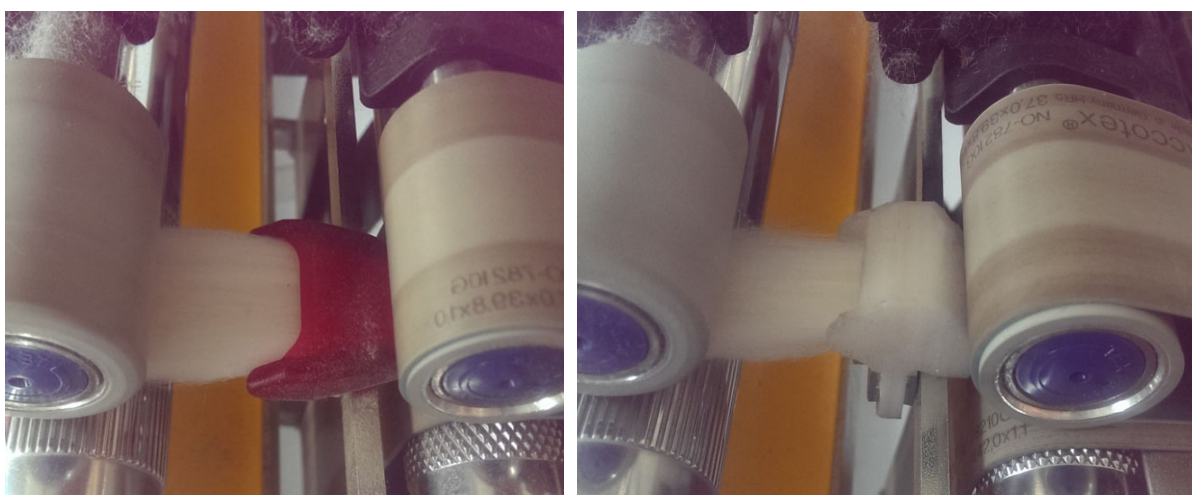
Figure 122 Pictures of conventional (left) and spiral (right) condenser integration
