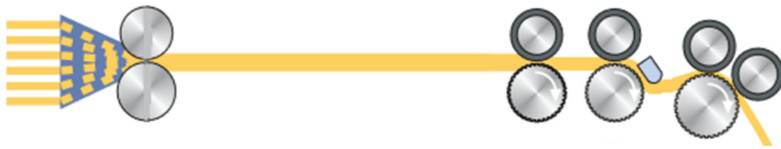
Figure 38 Principle of a Trützschler draw frame machine and its drafting arrangement
