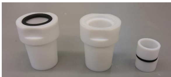
Figure 2.6. Teflon adaptors to use Schlenk tubes in the photoreactor.
