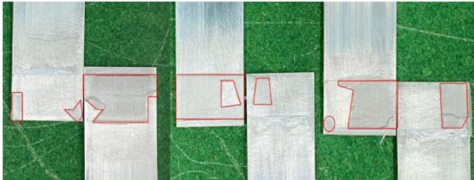
Figure 10.57. Tested plates after lap-shear tests for DGEBA_S4 where it can be seen not a cohesive failure in some of them but an adhesion failure.
