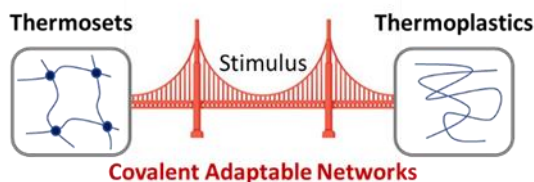
Figure 1.7. Representation of the boundary line between thermoplastics and thermosets thanks to CANs.
