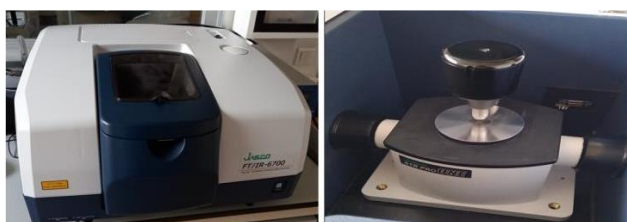
Figure 2.5. Jasco FT/IR-680 Plus spectrometer (left) and Specac Golden Gate ATR Teknokroma accessory in detail (right).
