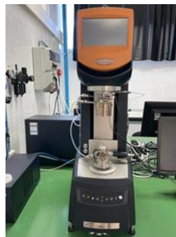
Figure 2.9. a) ARES G2 rheometer instrument and b) detail of the parallel plate geometry and the electrical heated plate.
