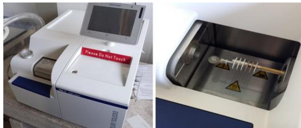
Figure 2.7. Mettler Toledo TGA 2 equipment (left) and detail of the furnace with the thermobalance (right).
