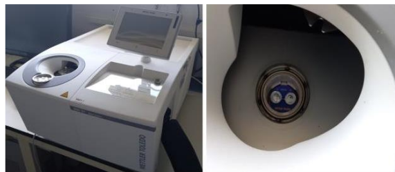
Figure 2.3. DSC 3+ device from Mettler Toledo (left) and zoom of its furnace (right).
