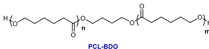
Figure 5.16. Structure of PCL-BDO .
