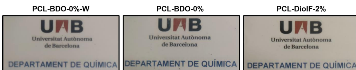
Figure 6.6. Photographs of the injected plaques of the single-component SS TPUs with the UAB logotype underneath.
