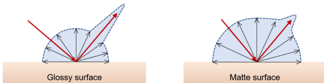
Figure 2.14. Schematic representation of glossy and matte surfaces according to the specular gloss.
