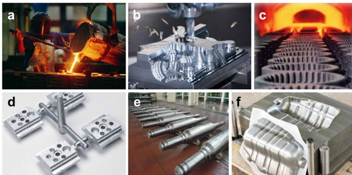
Figure 1.1. Traditional manufacturing methods. a) casting, b) machining, c) dies, d) drilling, e) turning, f) molding.
