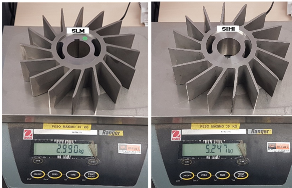
Figure 4.12. Weight comparison of SLM and SIHI impellers.
