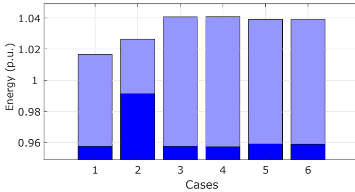
Figure 6.22: Maximum (light bars) and minimum (dark bars) total energy of the flexible dc-MMC for the six cases of normal operation (see Table 4.4).
