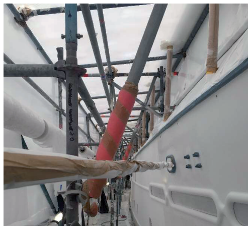
Figure S1. Example of a tent built around a vessel in the Mallorca shipyard, and the inside of the tent.
