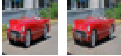
FIGURE 1.2: Reconstruction of an input images from the local gradients of a participating peer. Left: Original input images. Right: Reconstructed image from original gradients.
