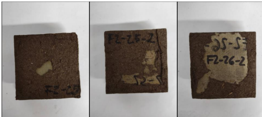
Figure A.18. Pictures of detached specimens during the internal bond test.
