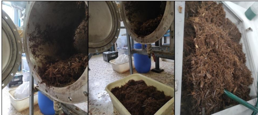
Figure 2.5. Pictures of exploded Arundo donax L. at different severities (increasing from left to right), during the drying.
