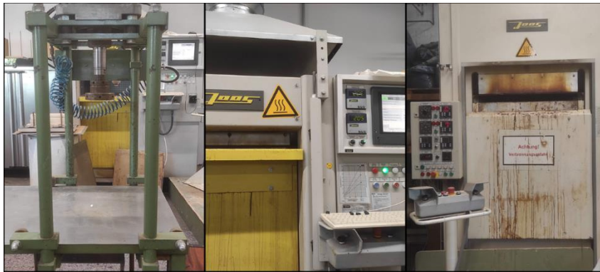
Figure A.11. Pictures, from left to right, of: Cold press, Joos LAP 40 hot press, and Joos HP-200 lab hot press (Chapter 6).
