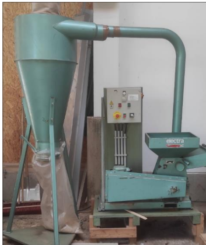
Figure A.5. Picture of the Electra hammer mill, used for grinding of steam exploded Arundo donax L. in Chapter 6.
