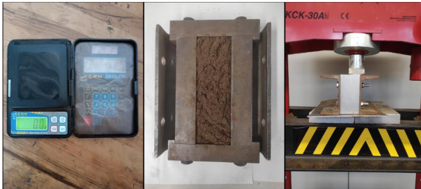
Figure A.8. Pictures of cold pressing process: weighing, mold preparation, and pressing.
