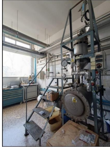
Figure A.2. Picture of steam explosion reactor and expansion chamber (Justinox company).
