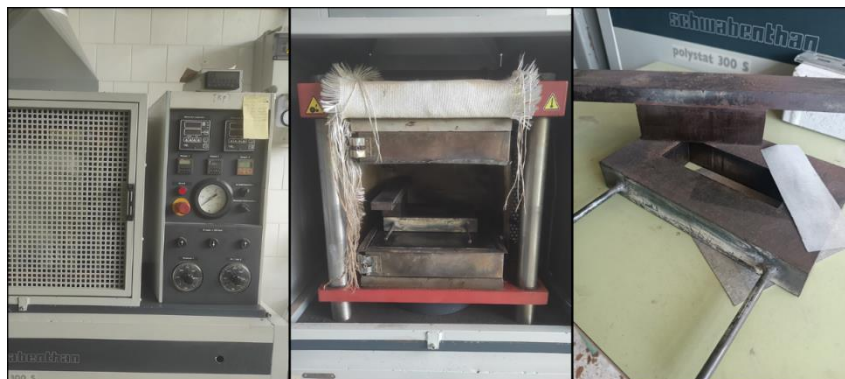
Figure A.10. Pictures of hot press and the mold used for manufacturing the specimens.
