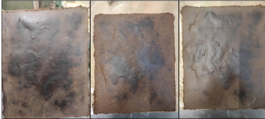
Figure 2.9. Picture of specimens after cold pressing (right), and after hot pressing (left).
