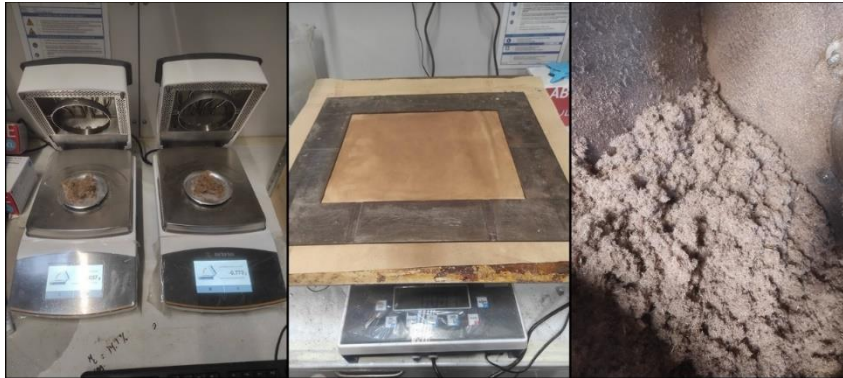
Figure A.7. Pictures of relative humidity measurement, weighting, and material inside the blender.
