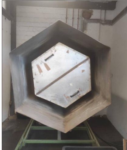
Figure A.6. Picture of the drum blender used for mixing the fibers with pMDI and water (Chapter 6).
