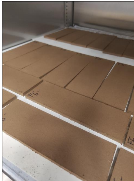
Figure 2.10. Picture of specimens being conditioned in the climatic chamber, after the cold pressing step.
