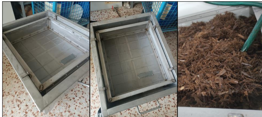
Figure A.3. Pictures of washing trolley and rinsing step.
