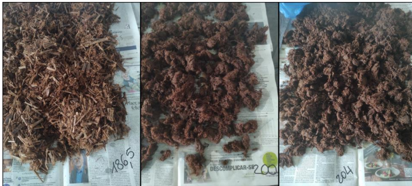
Figure 2.5. Pictures of exploded Arundo donax L. at different severities (increasing from left to right), during the drying.
