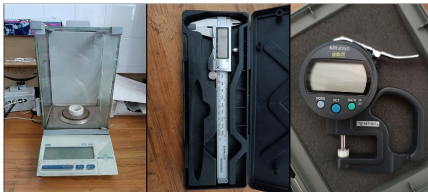
Figure A.19. Pictures of the precision scale, the digital scale, and the digital micrometer.
