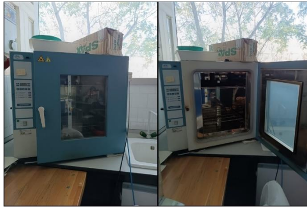
Figure A.13. Picture of electrical aerated stove JP Selecta SA (1600 W).
