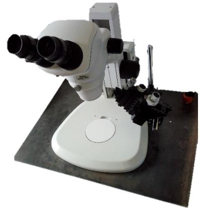
Figure VI-2. Microscope with holder for microsyringes on the right.
