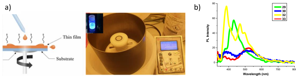
Figure 6.9. (a) Preparation of thin-films by spin-coating technique on Spectrosil B quartz substrates using compounds in THF, conc. 10^{-3} M. (b) PL emission spectra of acetylene precursors ( 29 and 32 ) and o -carborane containing compounds ( 30 and 33 ) in thin-films.
