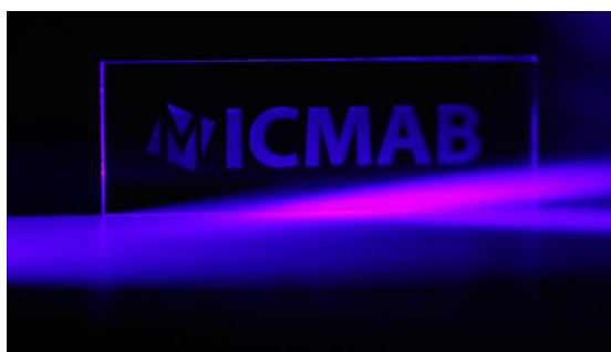
Fig. 3.12. Preliminary studies using thin films of 9 using DMP-2850 inkjet printer (Fujifilm) and the Molecular Gate S.L. technology, developed by Mariano Campoy-Quiles and Aleksandr Perevedentsev. 16
