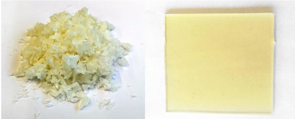
Figure 4.7: Left: Shredded polymer. Right: Injected plate.
