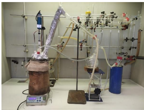
Figure 6.3: 1 Kg reactor assembly for polyester synthesis.
