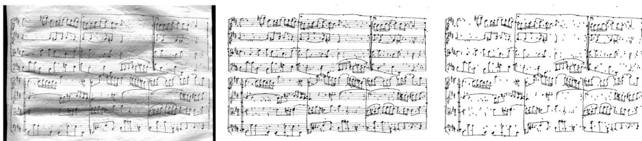
Figure 2.2: A music page, its binary image and the page without the staff lines. Reprinted from [49].
