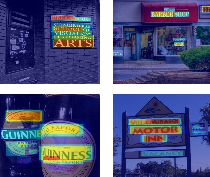
Figure 4.3: Heat maps obtained according to the confidence detection score of the predicted PHOCs.
