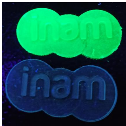
Figure 78. Logo of INAM 3D-printed with PIL3b formulation (up) with \text{CsPbBr}_3 NCs (2 wt%) (down) without PNCs. Picture taken under UV light.
