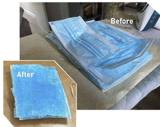
Figure 7. Processing surgical masks for transforming them into 3D printing materials. Photos Credits: University of Bristol, from reference [92]. Retrieved 27 January 2023.
