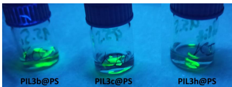
Figure 75. (Left) PIL3b@PS film, (centre) PIL3c@PS film, (right) PIL3h@PS film, immersed in a solution of potassium iodide (KI) in H 2 O (10 mg/mL) during more than 2 hours.
