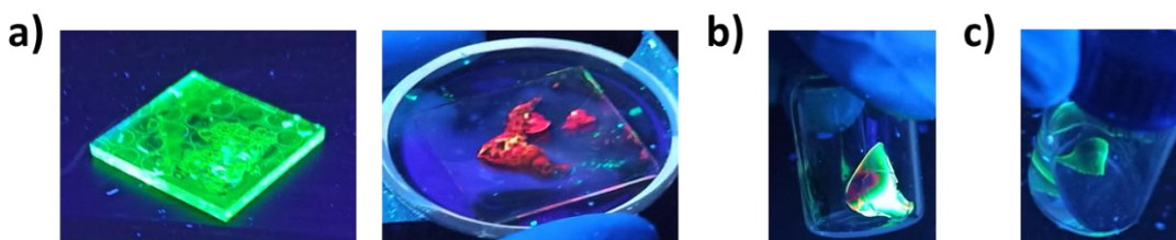
Figure 77. a) PIL3h@PS film on the surface of a glass, before and after dropping KI solution; b) Film prepared with 90 mol% of BA and 10 mol% of BDA after being 30 minutes into KI solution; c) Film prepared with 60 mol% of BA, 20 mol% of PEGDA and 20 mol% of BDA after being 10 minutes into KI solution.
