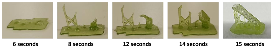
Figure 53. Evolution of Cu@PIL3.2 3D-printed stent modifying the exposure time.
