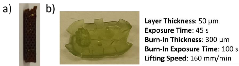
Figure 56. a) Cu@PIL3.2 stent treated at 160 °C for 30 minutes; b) Picture of Cu@PIL1.2 3D-printed base with the printing parameters.
