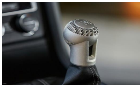
Figure 4. A printed part from a Volkswagen car using HP Metal Jet technology. Photo via HP, from reference [75]. Retrieved 20 November 2022.
