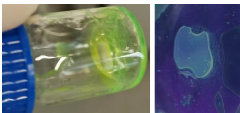
Figure 57. (Left) AcrEMA.N(CN) 2 -based photopolymer with 5 mol% of cross-linker (BDA) and CsPbBr 3 ; (right) the film formed after polymerisation. The absence of the green colour under UV illumination indicates that the PNCs are completely degraded.
