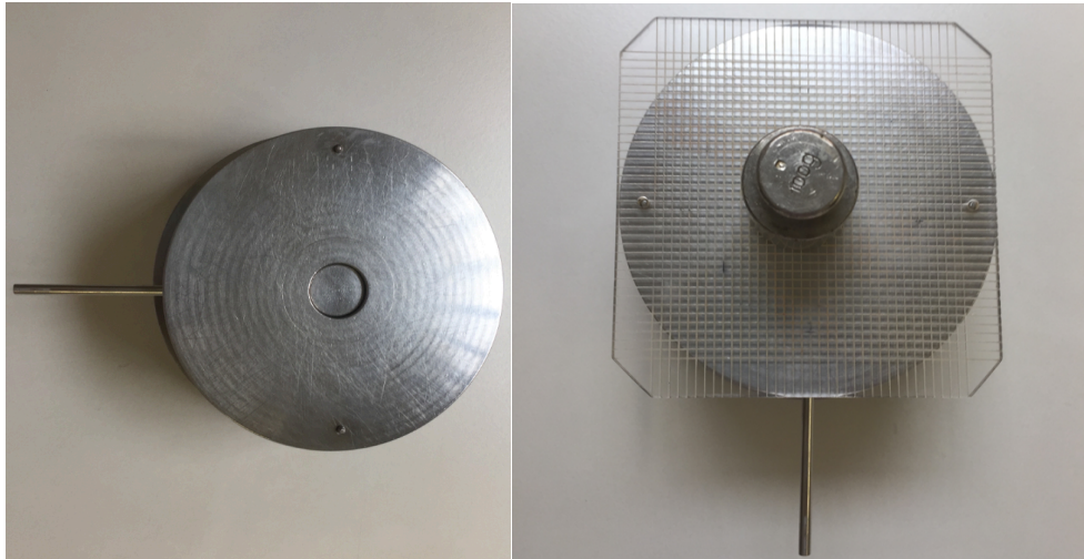
Figure 5-2. Extensometer designed by Dr. Alfonso del Pozo Ojeda and Dr. Josep Maria Suñé Arbussà. A) first position: cylinder has approximately 1 cm capacity volume. B) Second position: cylinder with no volume (even to the base) with the plastic coverage and 100 g weight.
