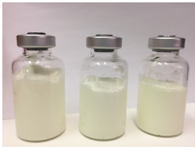
Figure 5-21. Stability of the bioadhesive emulsion 6-13 after 3 months storage at 5 °C, 25 °C and 40 °C.
