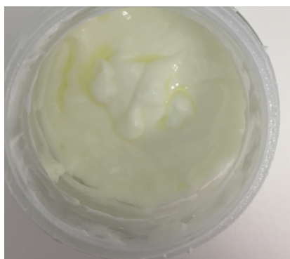
Figure 5-19: In-use stability the bioadhesive emulsion 6-13 after 3 months storage at 40 °C.
