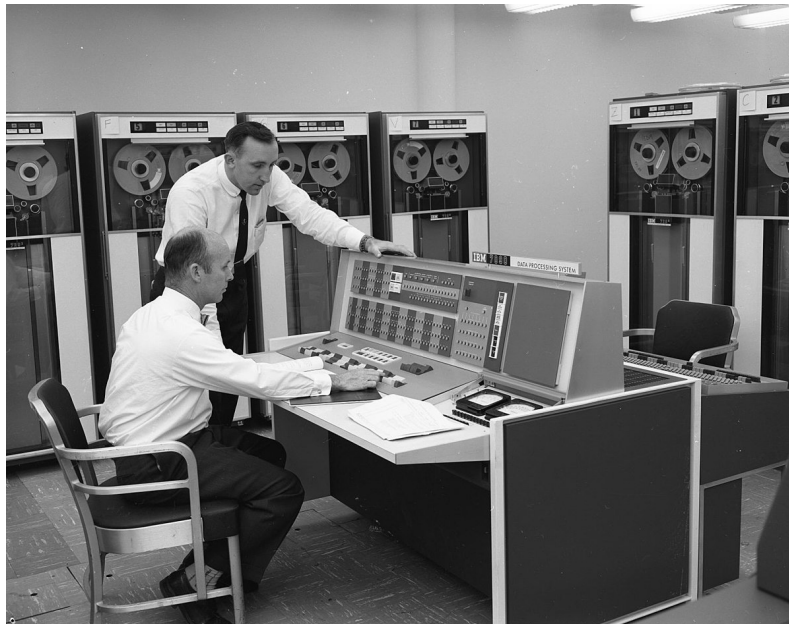
Figure 12. IBM 7090 machine. Computers didn't have a screen at the time, inputs had to be written in punch cards and outputs were printed on paper. From Wikipedia commons.
