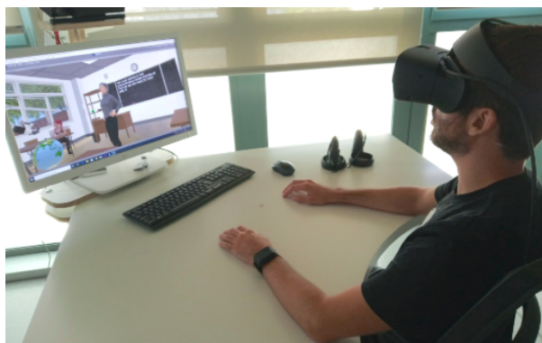
Figure 3.2: Setup of the experience. The user is wearing an Oculus Rift S headset and an Empatica E4 wristband. The computer screen allows observers to see what the user sees.
