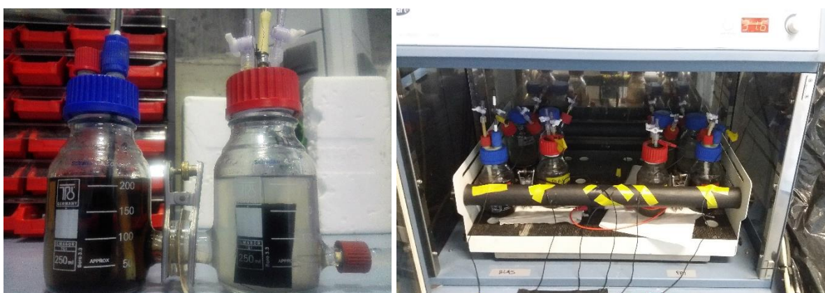
Figure S3. Reactors assembly and configuration in the orbital incubator.
