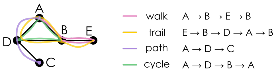
Figure 2.7: Examples of vertex sequences on a given graph including a walk (pink, repeating nodes and edges), a trail (yellow, unique edges but repeating nodes), a path (purple, unique nodes and edges) and a cycle (green, unique nodes and edges, closed path)
